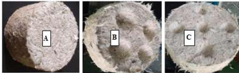
**Figure 1** Specimen: A. Flat Surface (FS); B. 4 Concaves Surface (CS4); C. 5 Concaves Surface (CS5)
