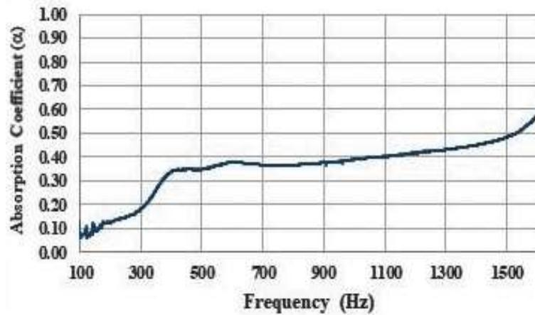
**Figure 9** Average absorption coefficients of 4 Concave surface (CS4) specimen
