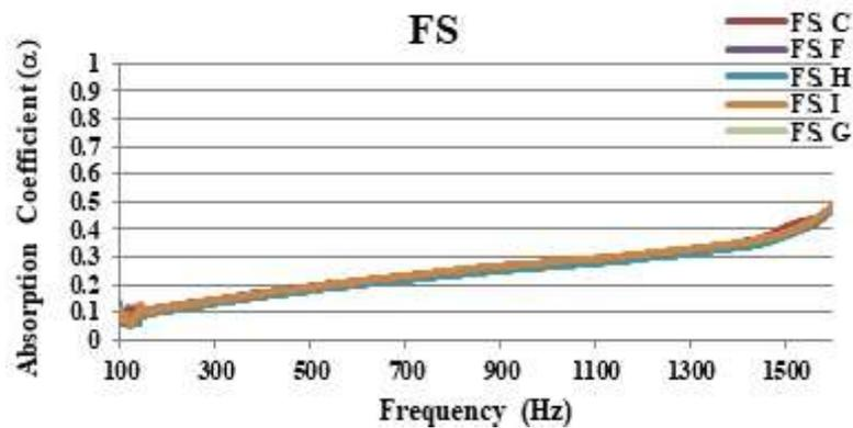
Figure 6. FS Absorption Coefficient Curve (C-F-H-I-G) sample
