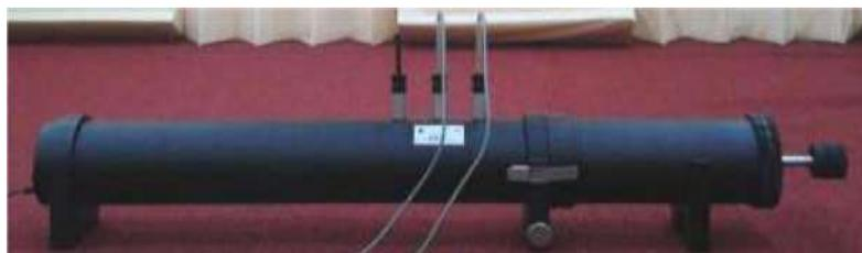
**Figure 2** Impedance tube type 4206
