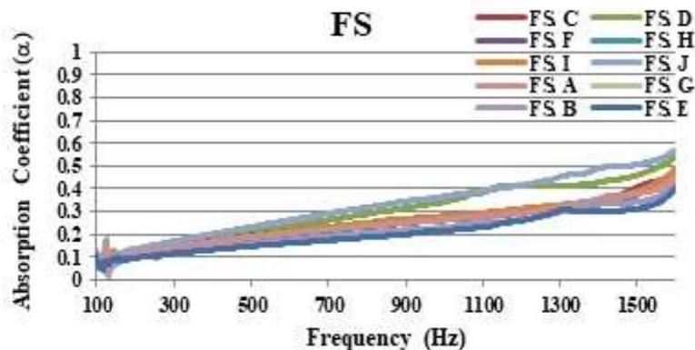
**Figure 5.** Absorption Coefficient of FS (A-J) samples
