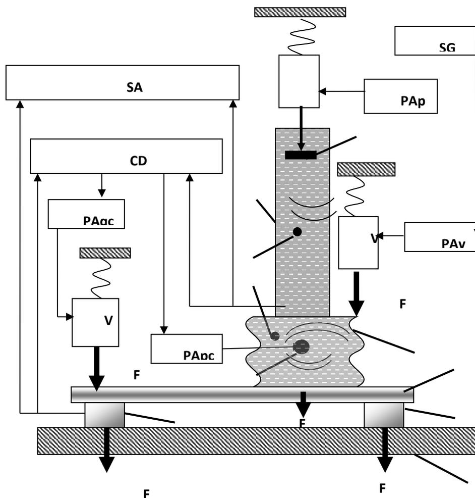
**Figure 3** Test bench of a two-channel AVS. CD - control device, PA - power amplifier, V - vibrator, SG - signal generator, SA - signal analyzer. Indices: c - compensation, p - pulsations, v – vibration
