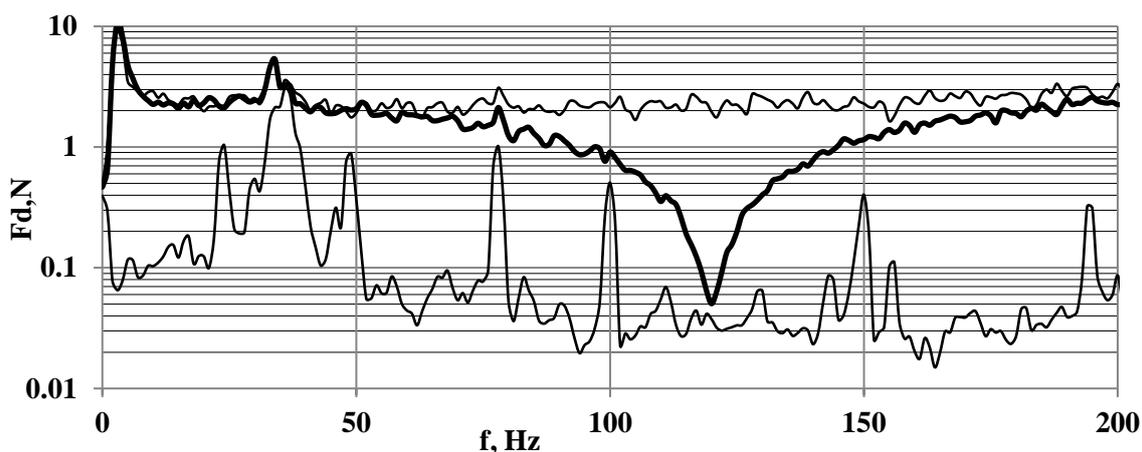
**Figure 4** Active damping by a resonator at 120 Hz. 1-initial signal, 2- damping, 3- disturbance
