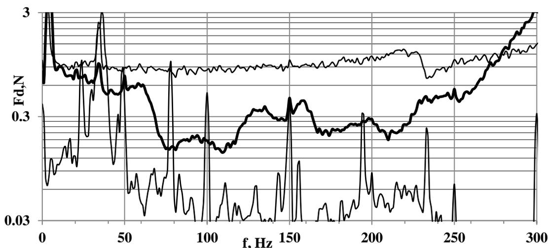
**Figure 5** Excitation by force and active damping by force. Elliptical filters  $\Delta f = 40-90$  Hz, filter order  $n = 1$ ,  $70-120$  Hz,  $n = 2$ ,  $100-180$  Hz,  $n = 2$ ,  $160-220$  Hz,  $n = 2$ ,  $200-260$  Hz,  $n = 2$ , the resonator is  $145$  Hz, phase  $0$ . 1- the initial signal, 2-damping, 3-disturbance
