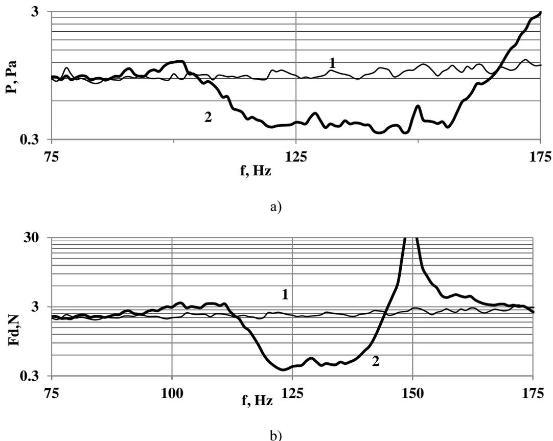
**Figure 7** Simultaneous excitation by pulsation and force. Combined damping by second-order elliptic filters of pulsation P in the range P110-160 Hz a) and the force  $F_d(f)$  in the range 120-140 Hz. b) . 1- initial signal, 2-damping.
