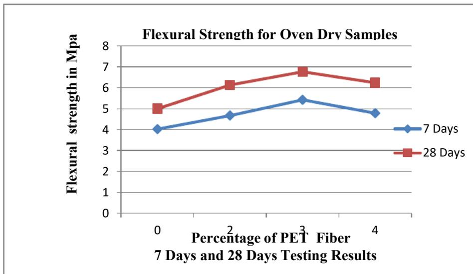
Graph 4 Flexural Strength for Oven dry curing samples
