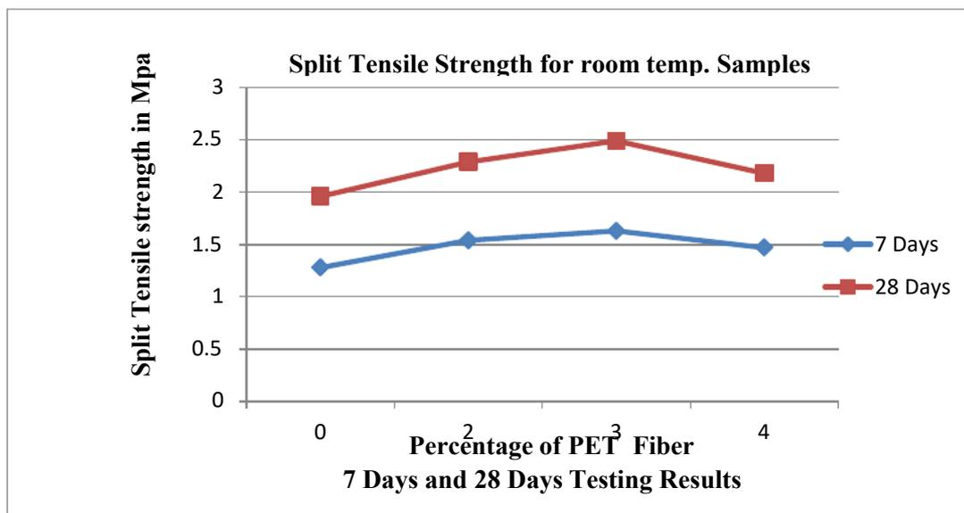
Graph 5 Split Tensile Strength for room temperature curing samples
