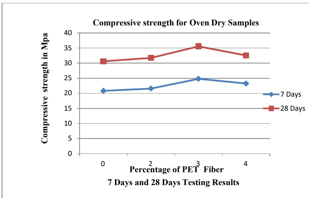
**Graph 2** Compressive Strength for oven dry samples
