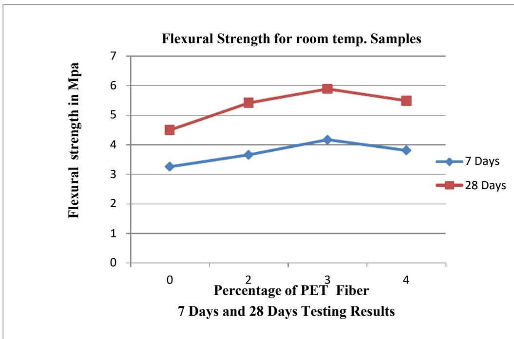
**Graph 3** Flexural Strength for room temperature curing samples
