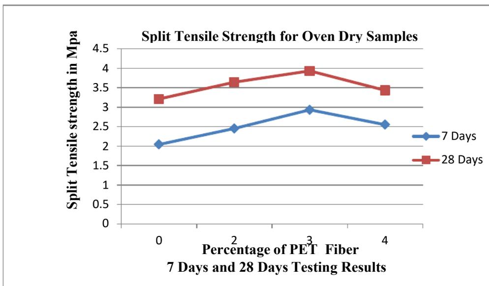
**Graph 6** Split Tensile Strength for Oven dry curing samples
