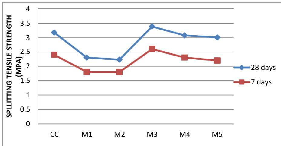
Figure 3 Split tensile strength test
