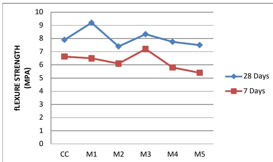
Figure 2 Flexural strength test results
