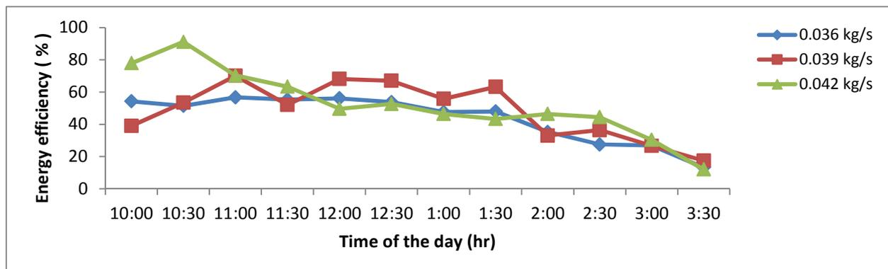
Figure 5. Variation of energy efficiency with time of the day at different mass flow rate
