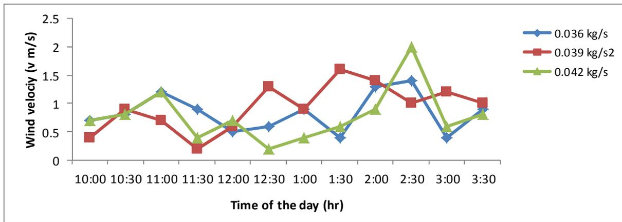
Figure 3. Variation of wind velocity with time of the day at different mass flow rate
