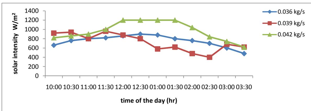
Figure 2. Variation of solar intensity with time of the day at different mass flow rate
