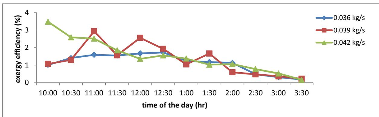
Figure 6. Variation of exergy efficiency with time of the day at different mass flow rate
