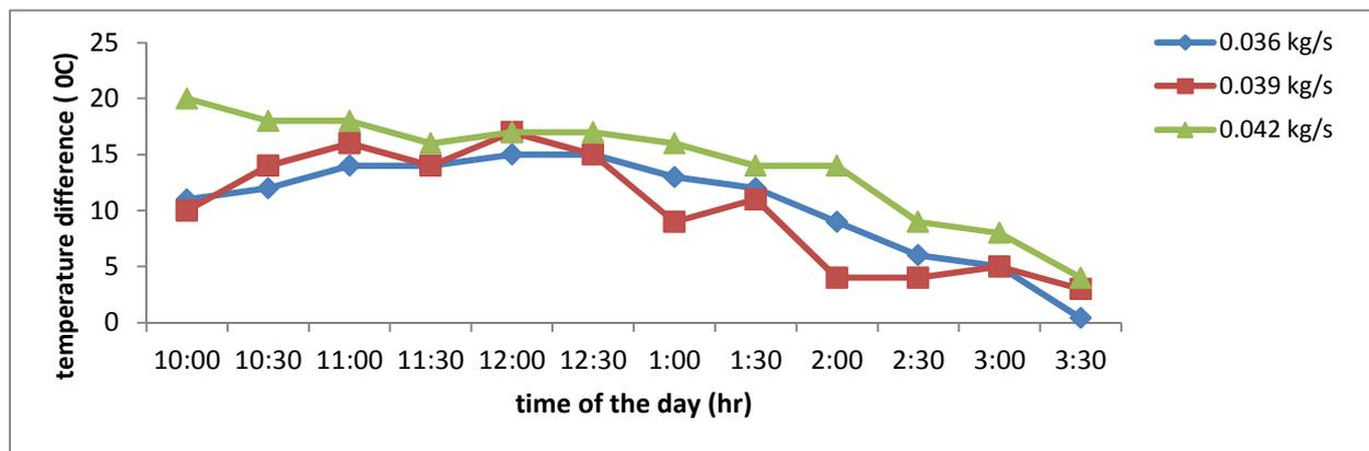
Figure 4. Variation of temperature difference between inlet and outlet with time of the day at different mass flow rate.
