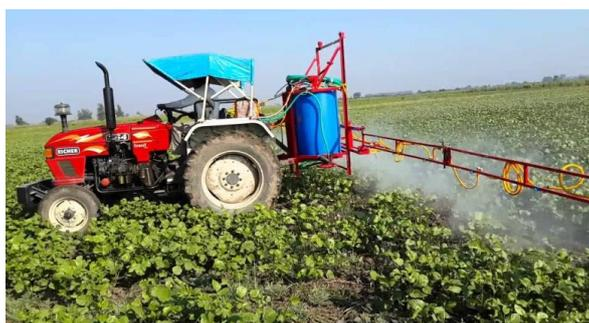
**Figure 4** Tractor Mounted Sprayer
