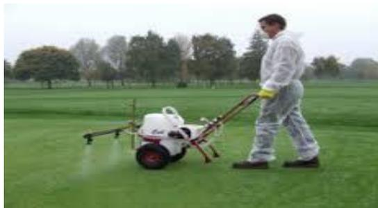
**Figure 3** Traction Sprayer
