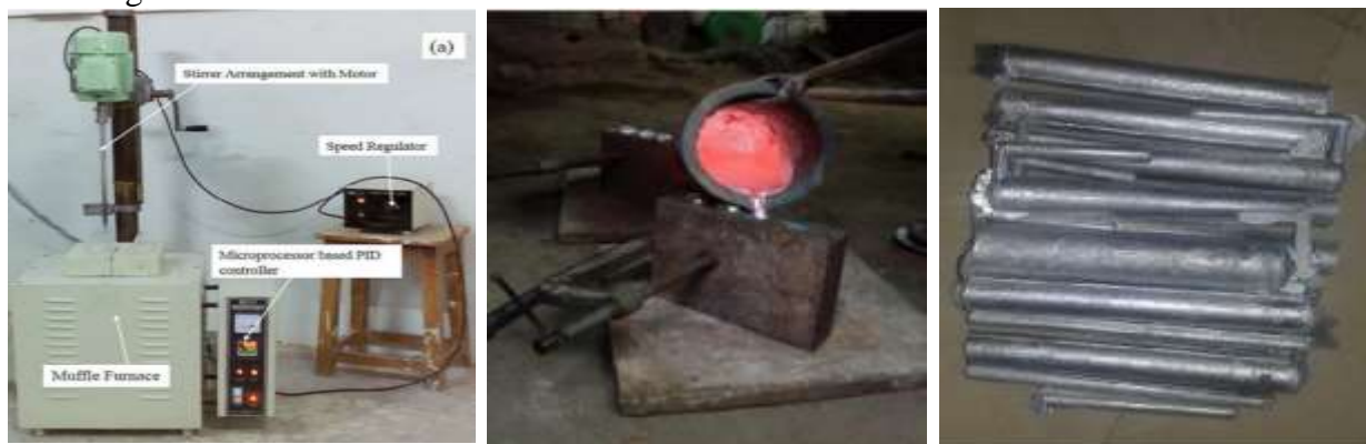
Figure 2 a. Stir Casting Set Up
