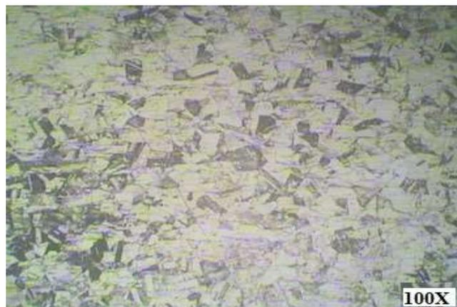
**Figure 2** Microstructure of the base material
