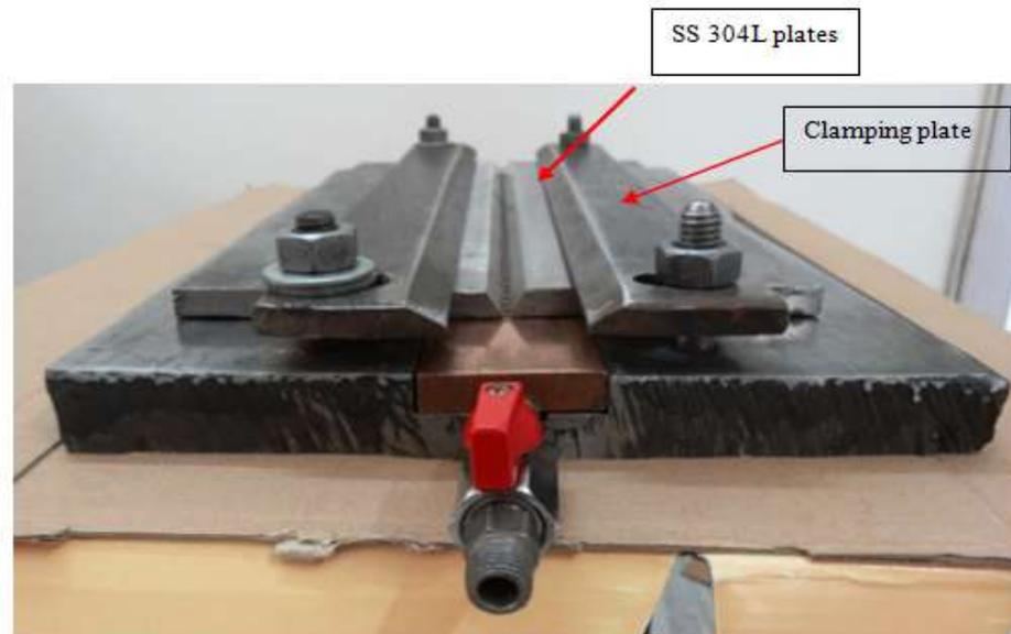
**Figure 5** Fixture with back purging arrangement
