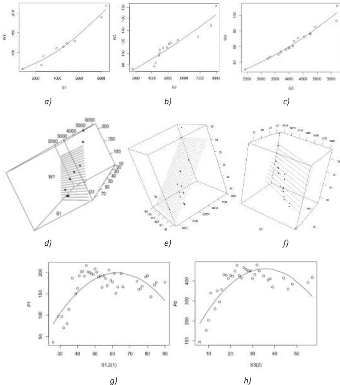
**Figure 4.** Filtered statistics and the resulting functional dependencies describing the operation of boilers and corrugated units: a) dependency  $W_1 = f(G_1)$ , b) dependency  $W_2 = f(G_2)$ , c) dependency  $W_3 = f(G_3)$ , d) dependency  $S_1 = f(W_1, G_1)$ , e) dependency  $S_2 = f(W_2, G_2)$ , f) dependency  $S_3 = f(W_3, G_3)$ , g) dependency  $P_1 = f(S_{1,2(1)})$ , h) dependency  $P_2 = f(S_{3(2)}(t))$ .
