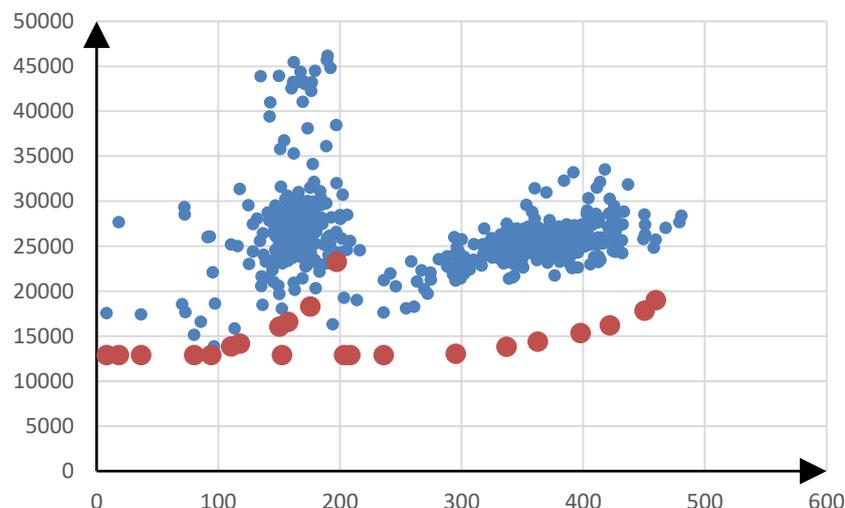
**Figure 6.** The dependence of the production volume on the price of resources used for it (gas and water for boilers): small blue dots mean retrospective data; big red dots mean the data obtained as a result of calculations on the model.
