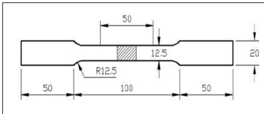
**Figure 3** Tensile specimen dimension
