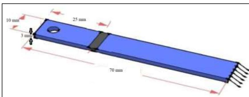
**Figure 5** Fatigue specimen
