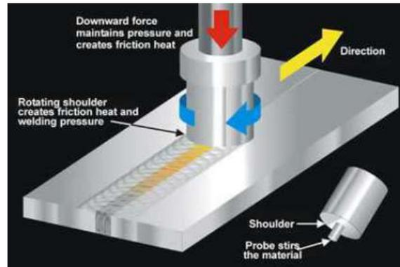
**Figure.1** working diagram of FSW
