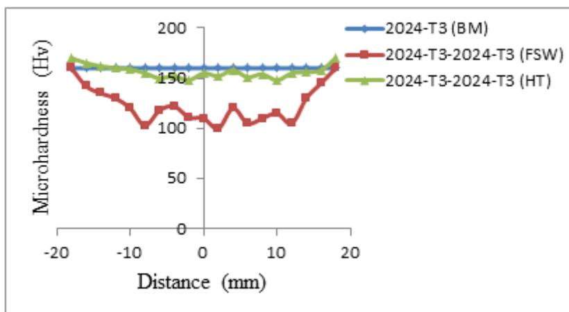
**Figure 4** The micro hardness values for the specimen.
