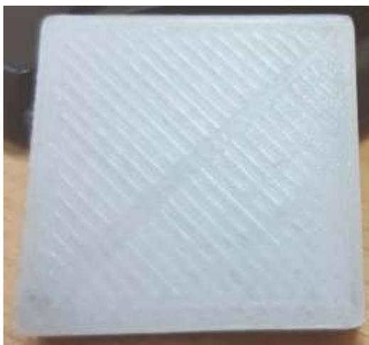
**Figure 12** Appearance of the test product surface printed of nylon
