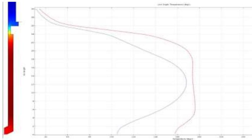
**Figure 9** Consolidated graph of temperature distribution at  $f = 19.5$  kHz,  $\alpha = 0$  (blue) and  $f = 121$  kHz,  $\alpha = 0$  (red). Heating time  $t = 4$  s
