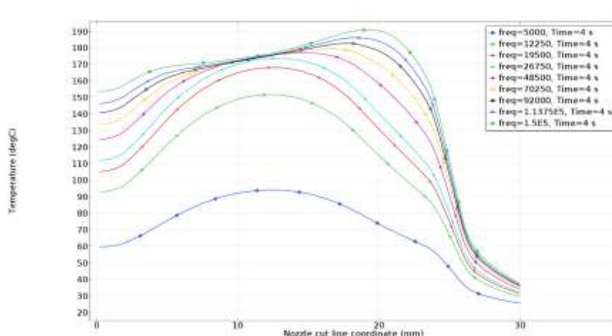
**Figure 6** Solution of thermal part of the parametric multi-physical task for  $f = 5.. 150$  kHz
