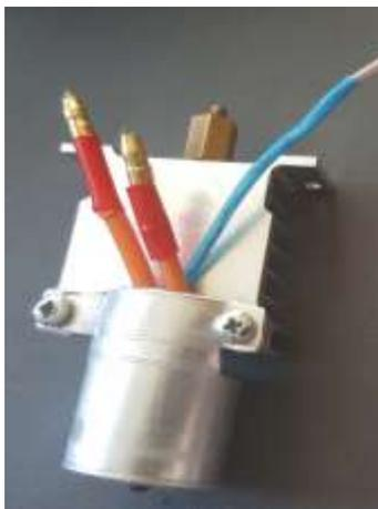
**Figure 10** Appearance of pilot extruder
