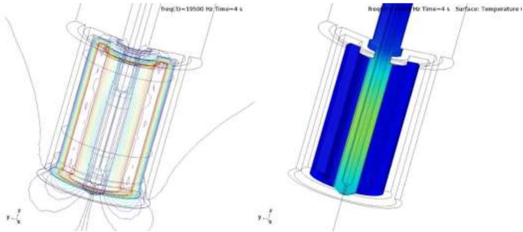
**Figure 3** Results of the electromagnetic and thermal tasks at  $f = 19.5$  kHz,  $t = 4$  s
