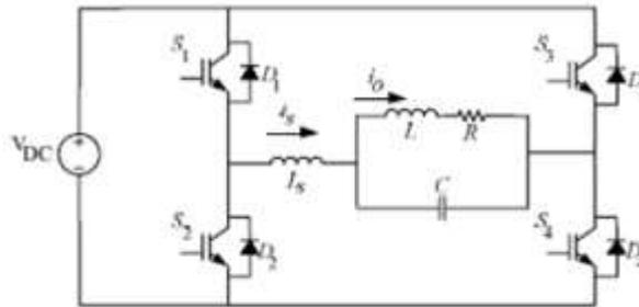
**Figure 1** Simplified circuit diagram of the induction heating power source
