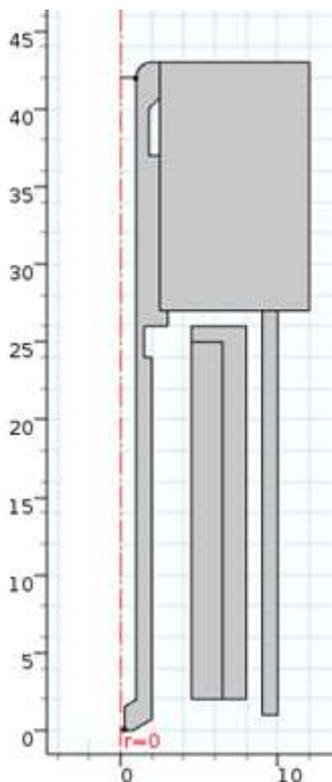
**Figure 2** Drawing of the induction heating system for FDM 3D nozzle
