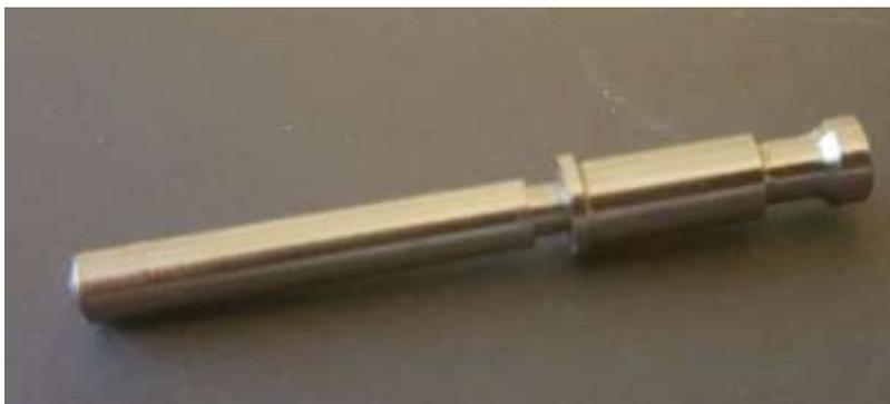
**Figure 11** Appearance of ferromagnetic nozzle
