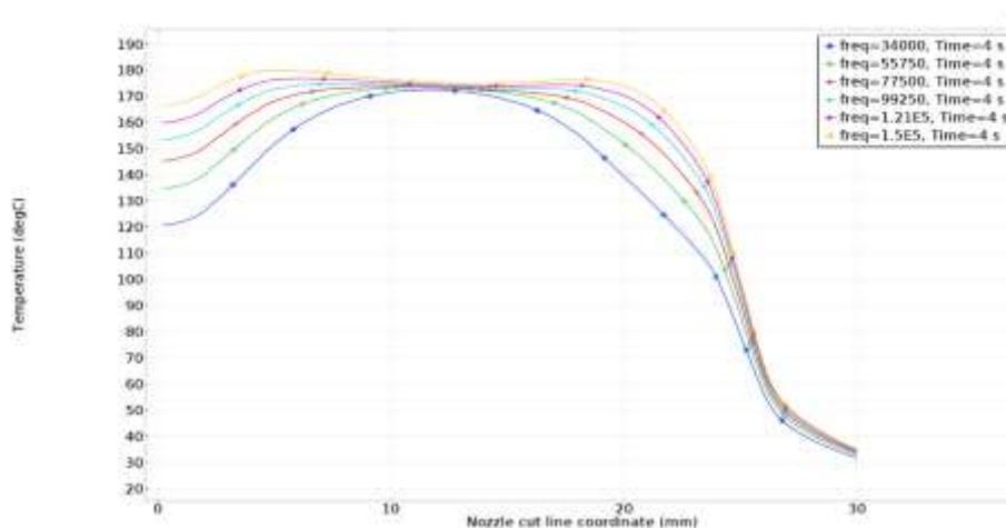
**Figure 8** Solution of thermal part of the parametric multi-physical task at  $f = 34.. 150$  kHz,  $\alpha = 1^\circ$
