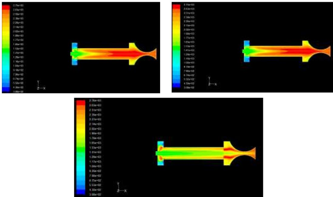
**Figure 4** Contours of static temperature for 50,80,110,140 and 170m/s
