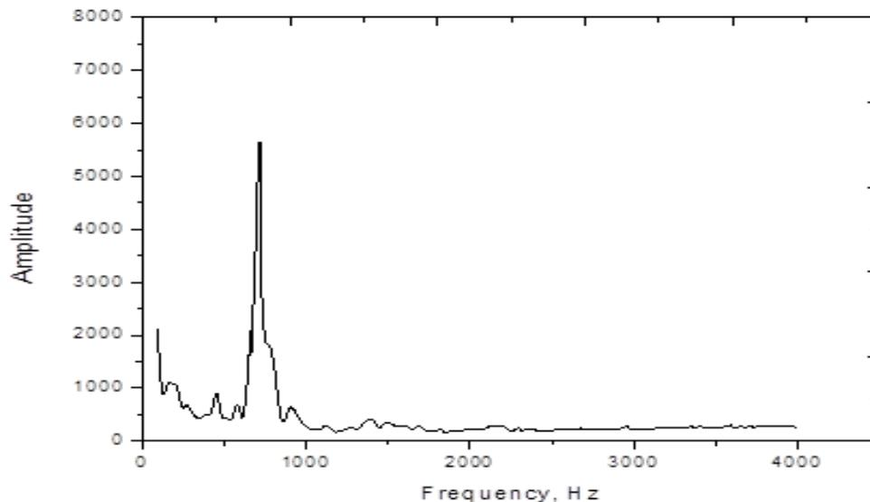
**Figure 3** Fast Fourier transform (FFT) plot for turbulent flow at 1700 lpm flow rate
