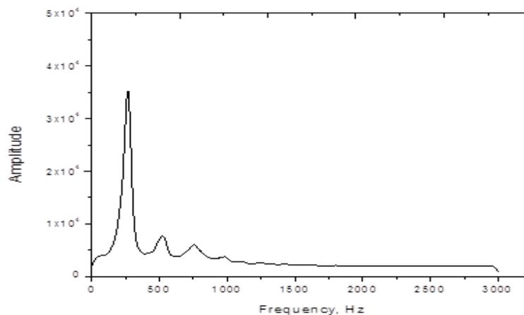
**Figure 2** fast Fourier transform (FFT) plot for laminar flow at 700 lpm flow rate
