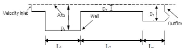
**Figure 1** Computational model of SRM cavity
