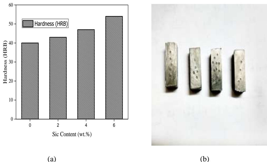
**Figure 3** (a) Hardness variation with wt. % of SiC contents (b) Specimens of hardness Test
