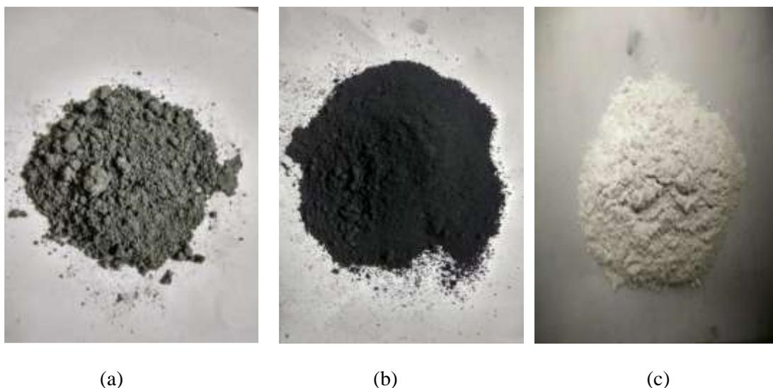
**Figure 1** (a) SiC particle (b) Gr particle (c) MD Particle
