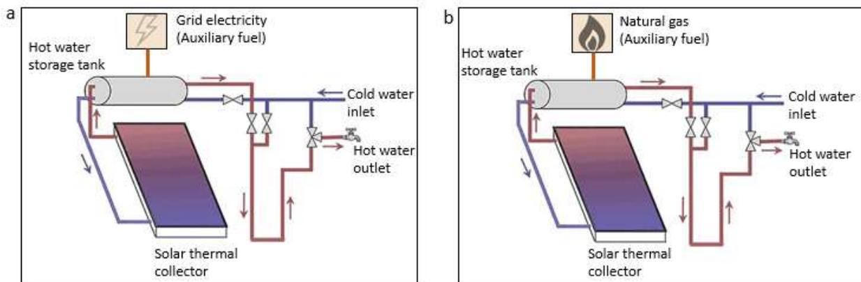
**Figure 1** a) Electric boosted solar water heater; b) Natural gas boosted solar water heater.
