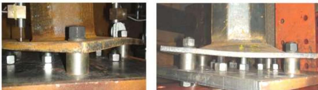
**Figure 11** Deflected shape of flange under maximal load
