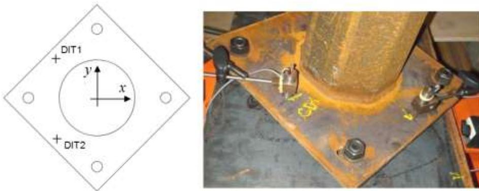
**Figure 5** Displacement inductive transducers DIT1 and DIT2 positions
