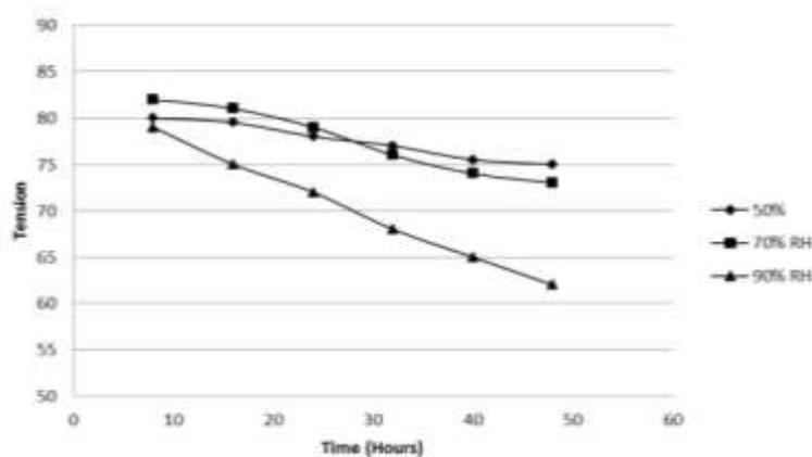
**Figure 5** The decrease in tension for all three *kompang* during experiment.
