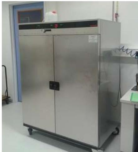
**Figure 2** Three samples was exposed to humidity in Memmert Climate Chamber HPP 750.
