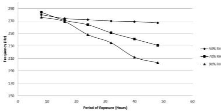
**Figure 7** Frequency reduction of the membrane after 48 hours of exposure
