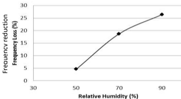
**Figure 8** Frequency reduction on kompang after 48 hours of exposure to different humidity.
