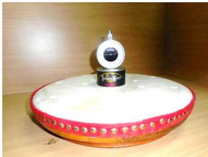
**Figure 3** Tension measurement using Tama Tension Watch.
