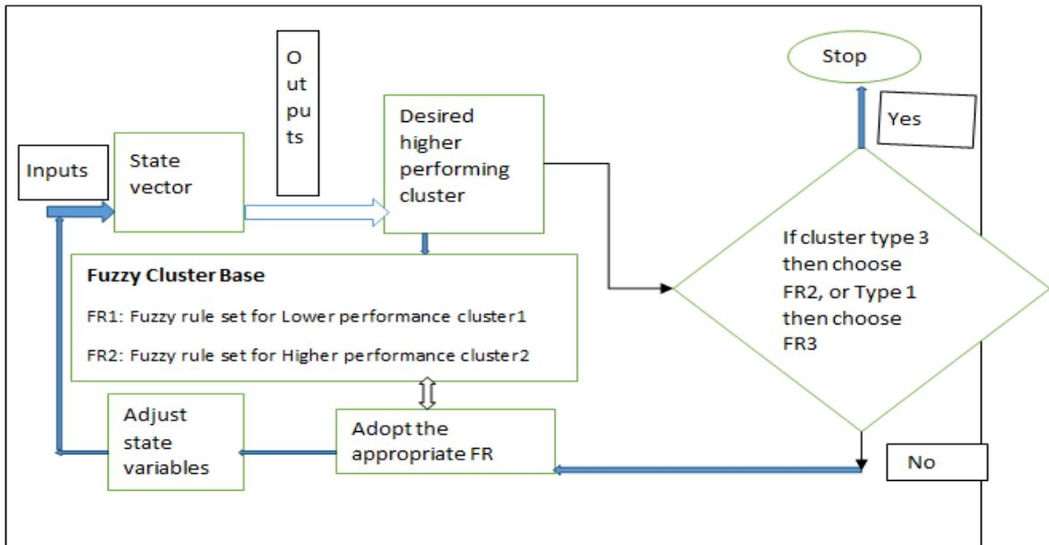
Figure 4 MANET system model controller for Packet Delivery Ratio (PDR)
