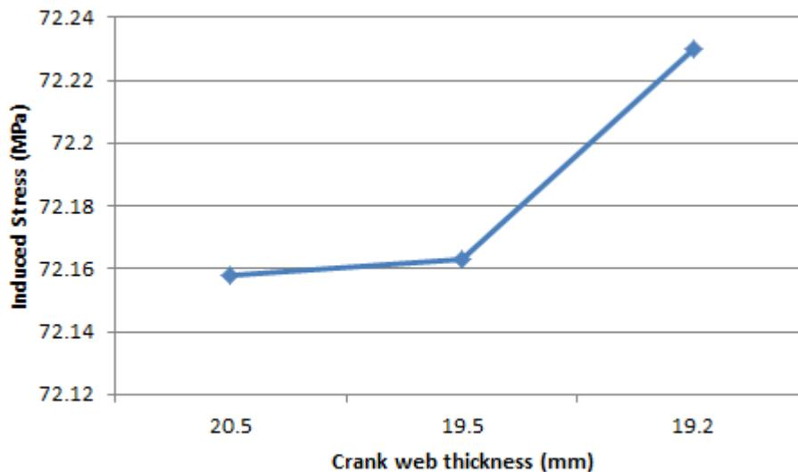
**Fig 4.1** Induced stress with crank web thickness
