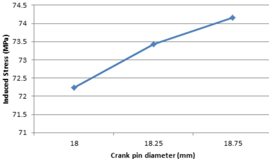
**Fig 4.2** Induced stress with Crank pin diameter
