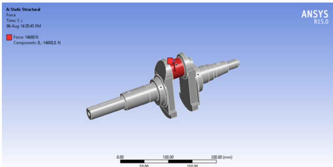
**Fig 3.4** Load applied on Crankpin of Shaft
