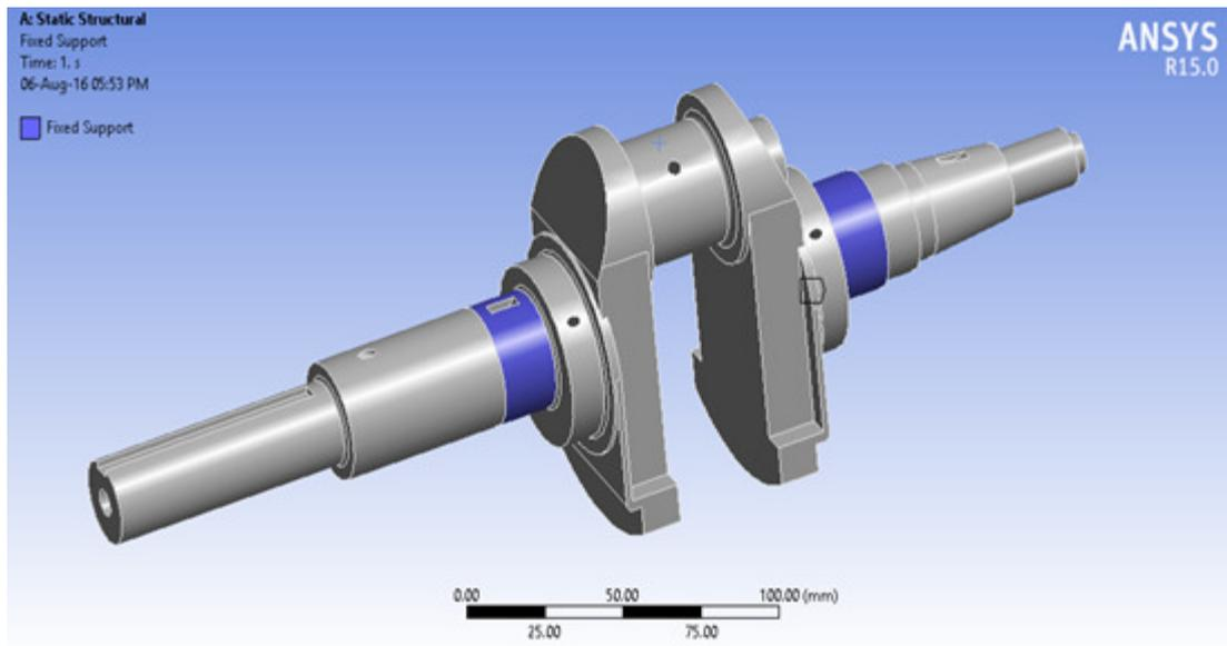
**Fig 3.3** Boundary conditions of Crankshaft
