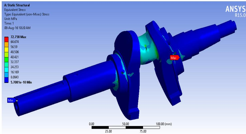
**Fig 3.5** Von-mises stress at cranweb thickness 20.5mm
