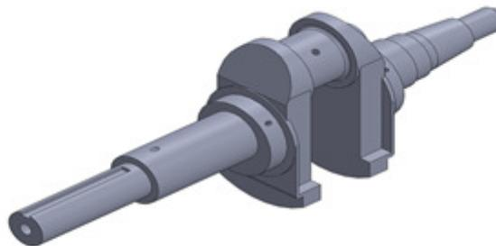
**Fig 3.1** Model of Single Cylinder Crankshaft Drawn by Solidwork
