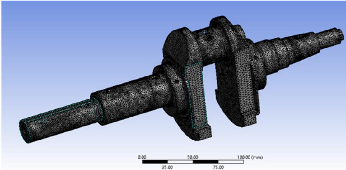
**Fig 3.2** Meshed model of Crankshaft
