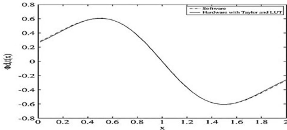
Fig. 6. The Wavelet Function using the first Derivative of the Gaussian function and its Hardware Approximation with Taylor and LUT..
