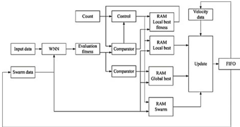
Fig. 8 The Block Diagram of the Hardware Implementation for PSO Algorithm.
