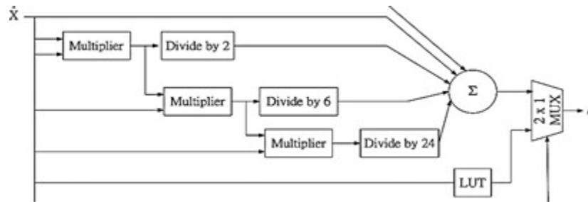
Fig. 5. The Overall Component of the Wavelet Layer Using the First Derivative of the Gaussian Function.
