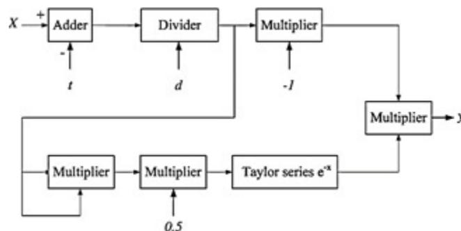
Fig. 4. The Block Diagram of the Hardware Implementations of the Euler Function.
