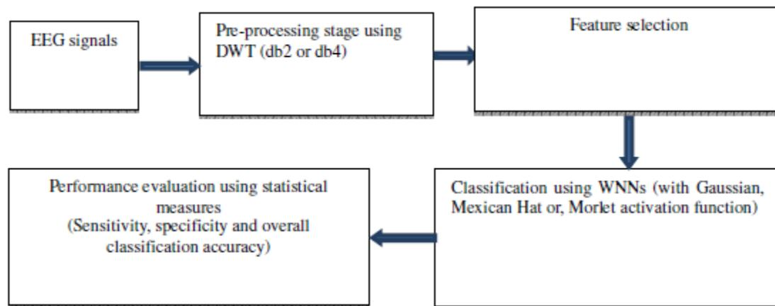
Fig. 1. Block Diagram for the WNN Based Epileptic Detection
