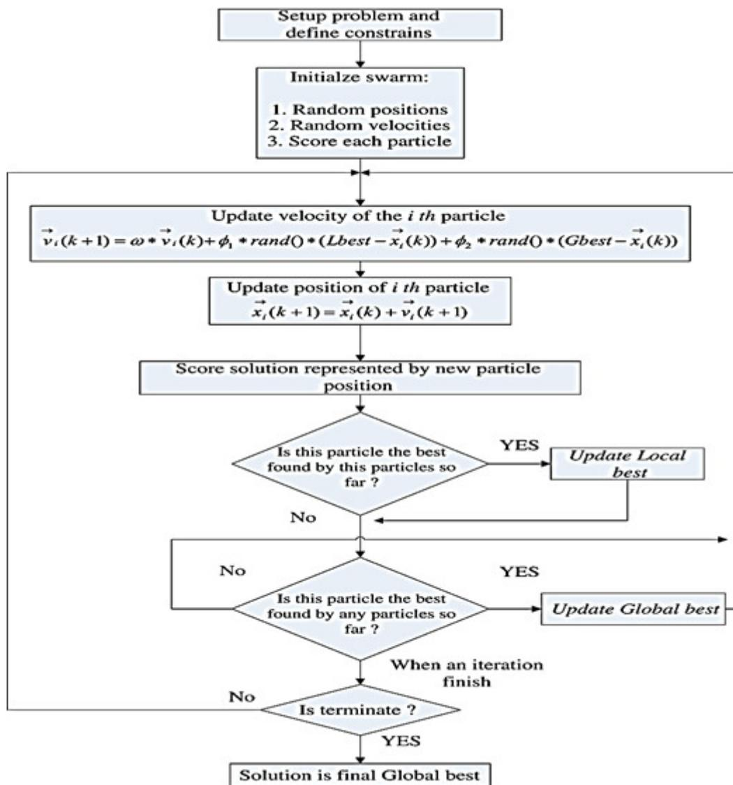
Fig. 2. PSO Algorithm Flowchart to Illustrate The Steps and Update Equations
