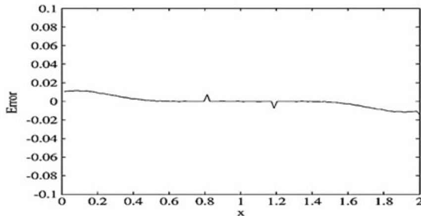
Fig. 7. The Error Curve of the Reference Function (the first derivative of the Gaussian function) and Approximated Function.
