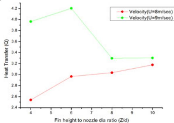
**Fig-20:**  $Z/d$  to heat flux ( $Q/A=W/m^2$ ).
