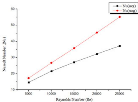
**Fig-16:** Effect of Reynolds number on Nusselt number. **Fig-17:** Effect of Reynolds number on temperature.
