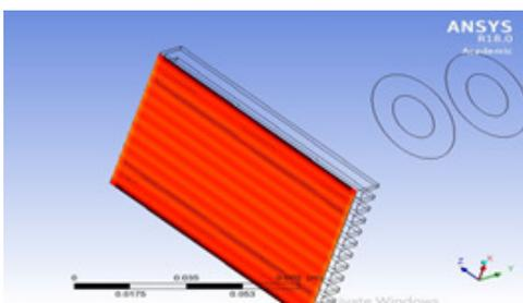
**Fig-10:** Variation of temperature on fin base.
