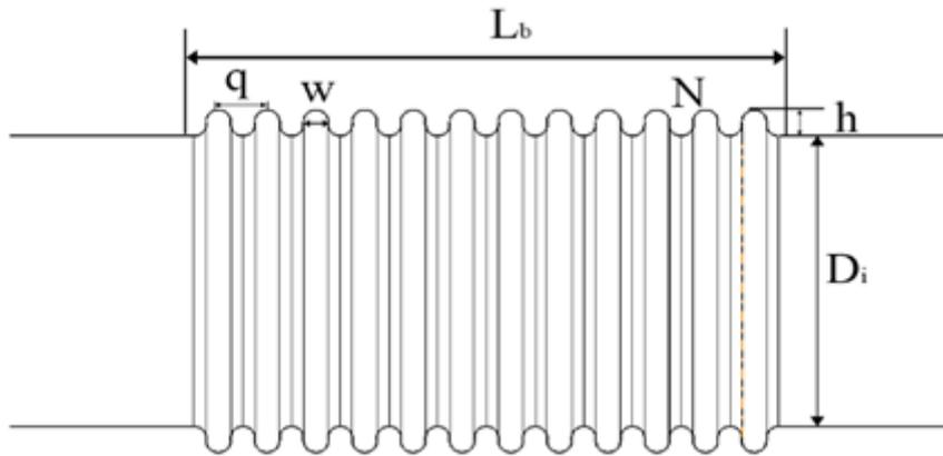
**Figure 2** The factor of bellows
