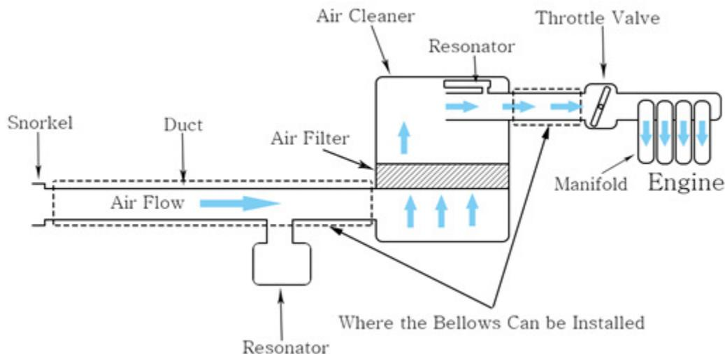
Figure 1 Simple diagram of the intake system
