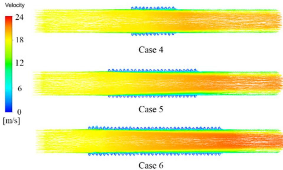
**Figure 5** Velocity vector with the change in number of bellows for each case
