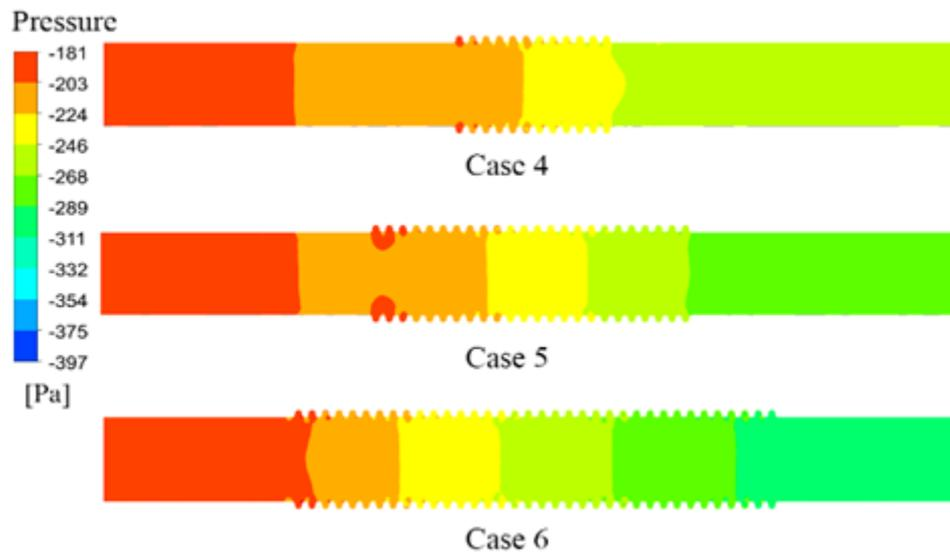
**Figure 5** Pressure change following the change of number of bellows
