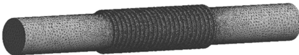
**Figure 3** Mesh creation of bellows
