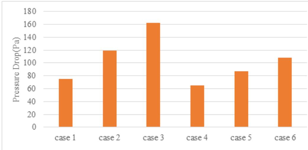
**Figure 4** Pressure loss graph in accordance with the change of number of bellows
