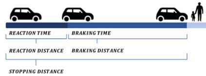
**Figure 3** Illustration of stopping distance
