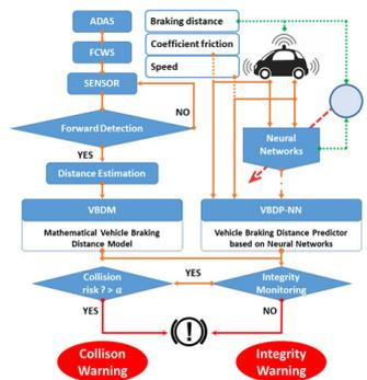
**Figure 4** Block diagram of reinforced FCWS constructed by VBDP-NN
