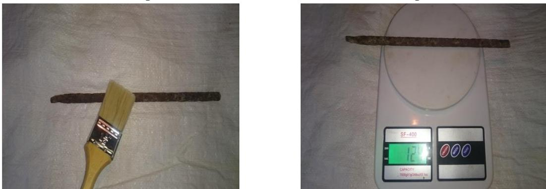
**Figure 4** The processes of cleaning and weighing of steel bar
