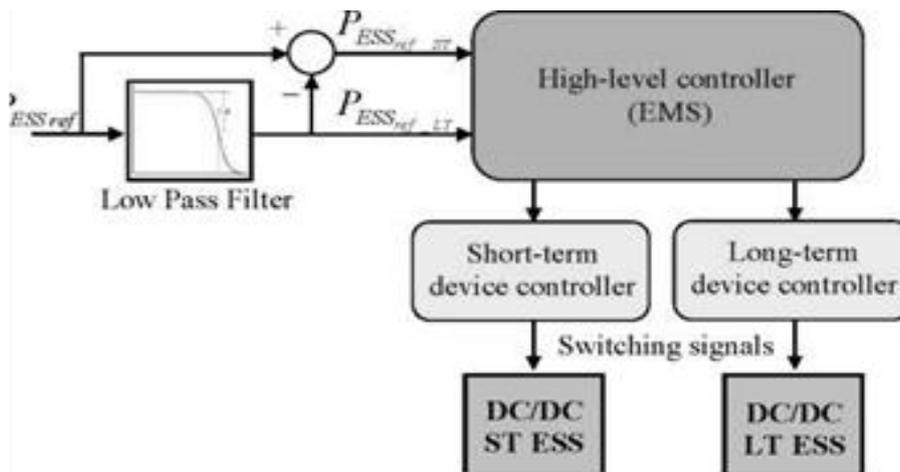
Figure 8 Example of energy management using linear filtering [10]
