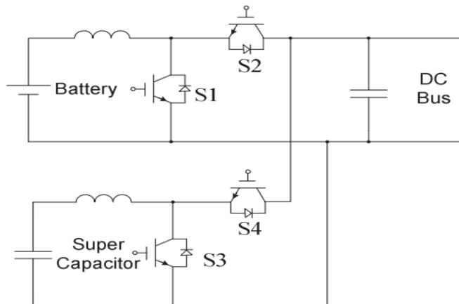
**Figure 2** Bidirectional buck/boost converter with common dc bus [3]
