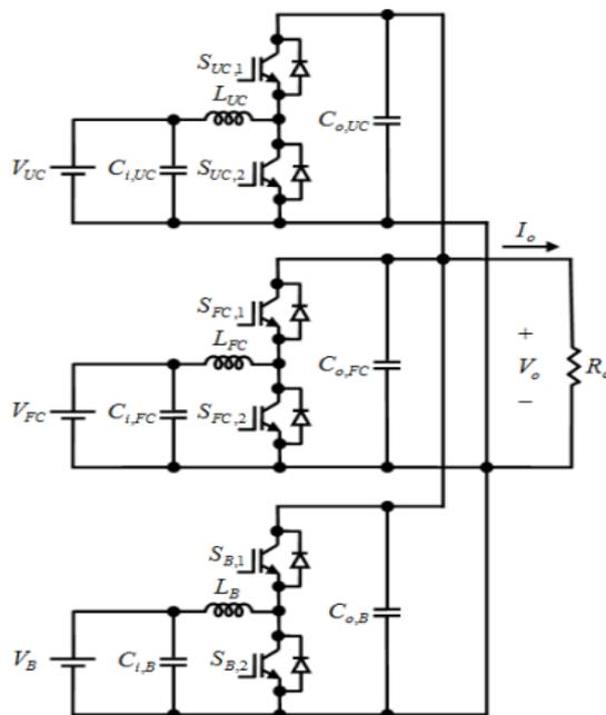
Figure 5 Bidirectional multi-port dc-dc converter [6]
