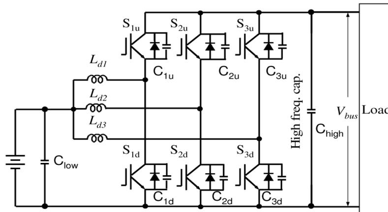
Figure 4 Bidirectional three-phase interleaved dc-dc converter [5]
