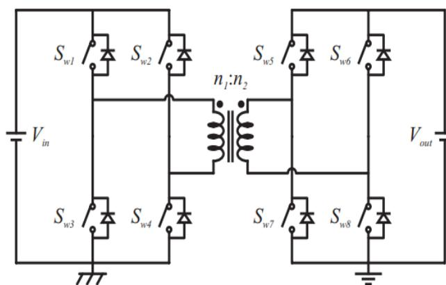
**Figure 3** Bidirectional full-bridge dc-dc converter [4]
