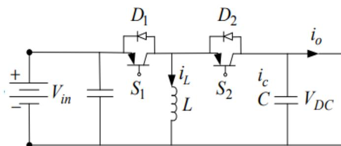
**Figure 1** Circuit diagram of the bidirectional dc-dc buck-boost converter [2]
