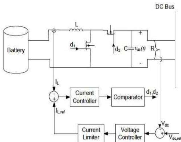
**Figure 6** Synchronous buck converter with current-mode control [7]
