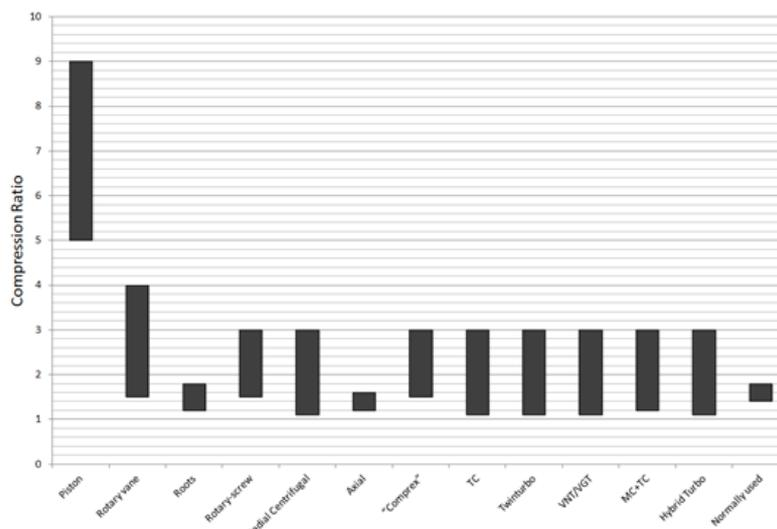
**Figure 3** Comparison of supercharging systems by a compression ratio
