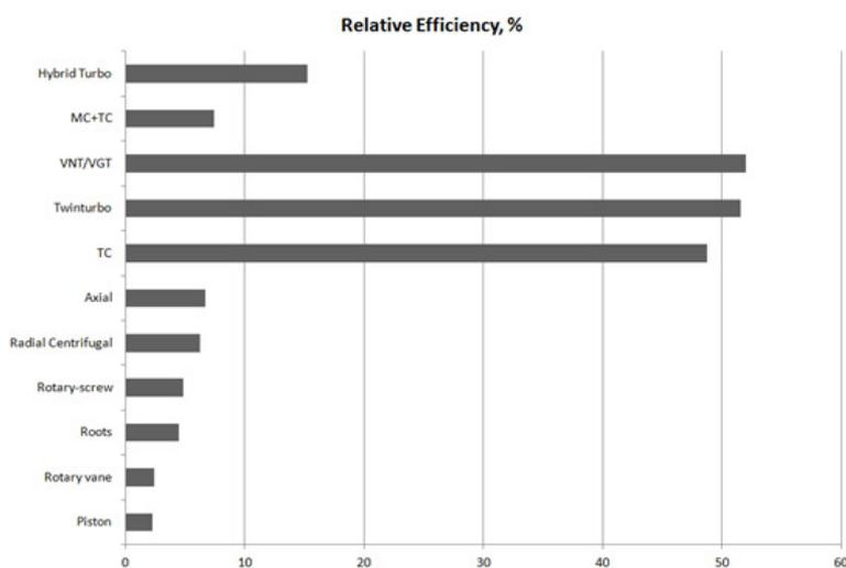
**Figure 4** Comparison of boost systems by relative efficiency
