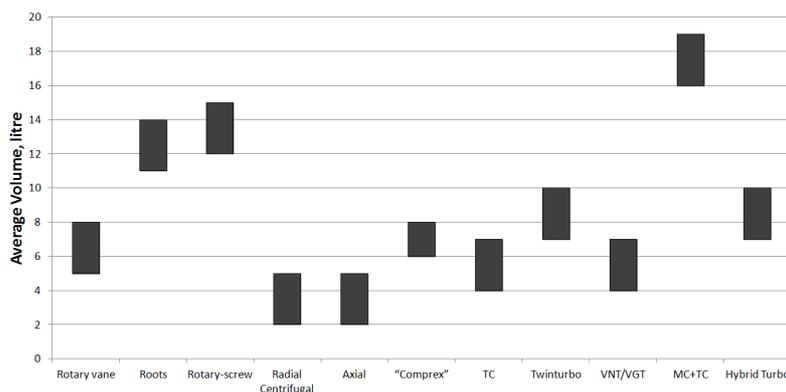
**Figure 1** Comparison of supercharging systems in terms of overall dimensions
