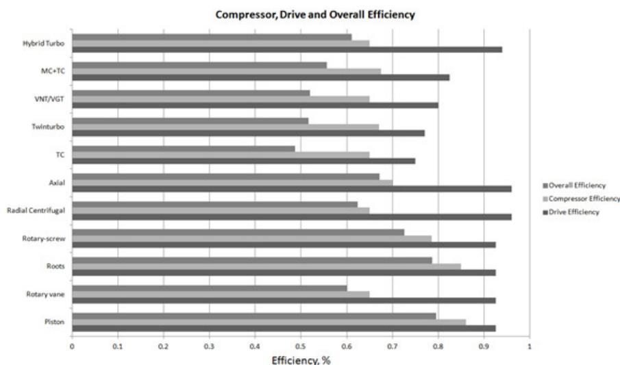
**Figure 2.** Comparison of boost systems by efficiency
