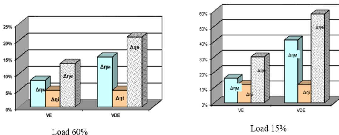
**Figure 9** Increase the efficiency of engines with adjustable working volume and/or compression ratio.
