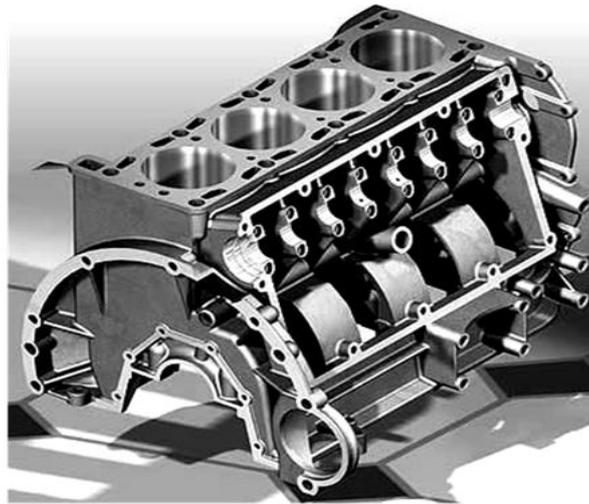
**Figure 7** The cylinder block of traverse engine
