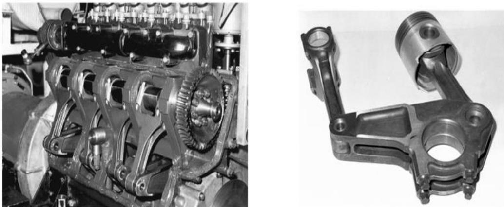
**Figure 3** Traverse diesel T-01 ( $iV_h = 9,1$  l) and its movement details based on the YaMZ-8424 engine
