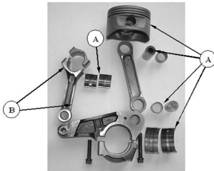
**Figure 6** Details of the conversion mechanism of the traverse engine: A - standard parts; B - additional parts (manufactured according to standard technologies and from traditional materials)
