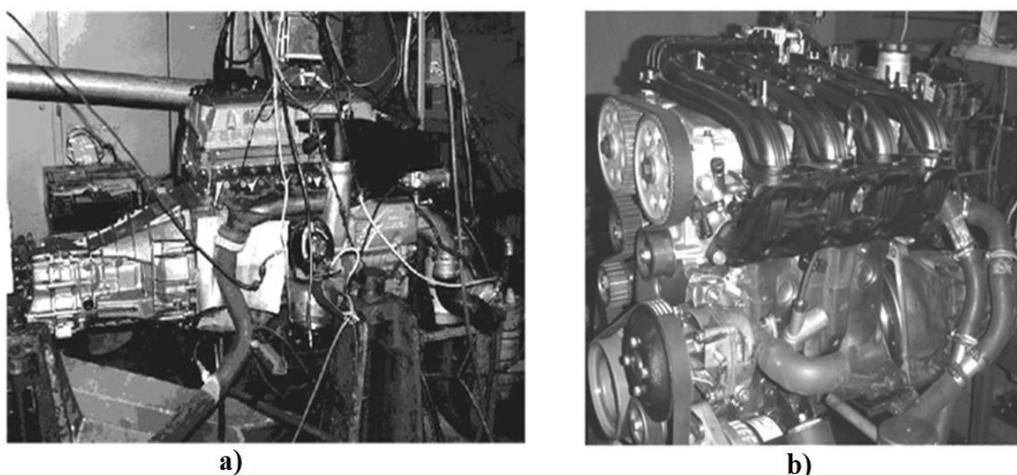
**Figure 4** Traverse engines with spark ignition: a) - VE111 ( $iV_h = 2$  l) on a DaimlerChrysler engine M111 base, b) - VAZ 11194VE ( $iV_h = 1.4$  l) based on VAZ 11194 engine
