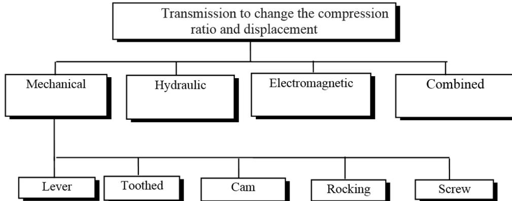
**Figure 1** Classification of gears and mechanisms for regulating the compression ratio and working volume
