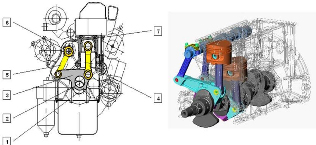
**Figure 5** Traverse mechanism of NAMI engines
