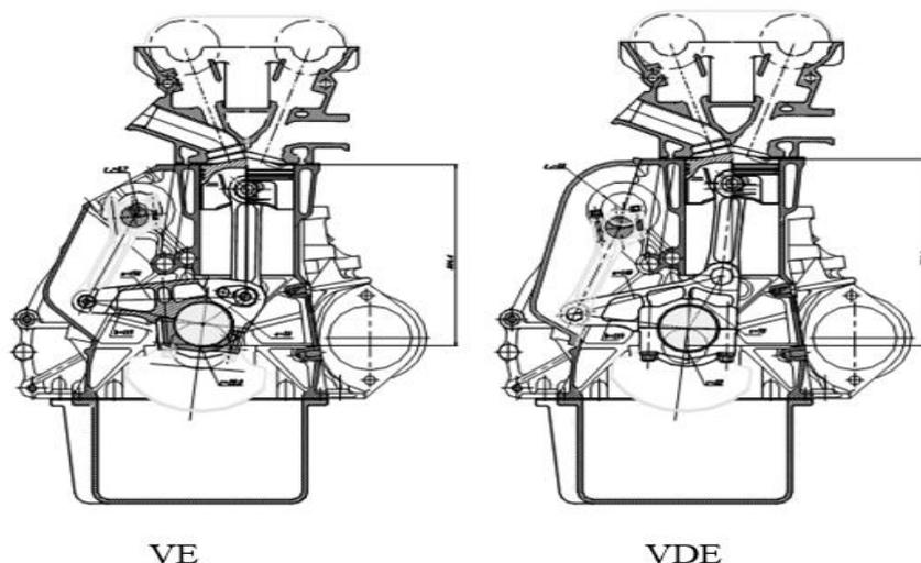
**Figure 8** Cross sections of engines with adjustable working volume and/or compression ratio.
