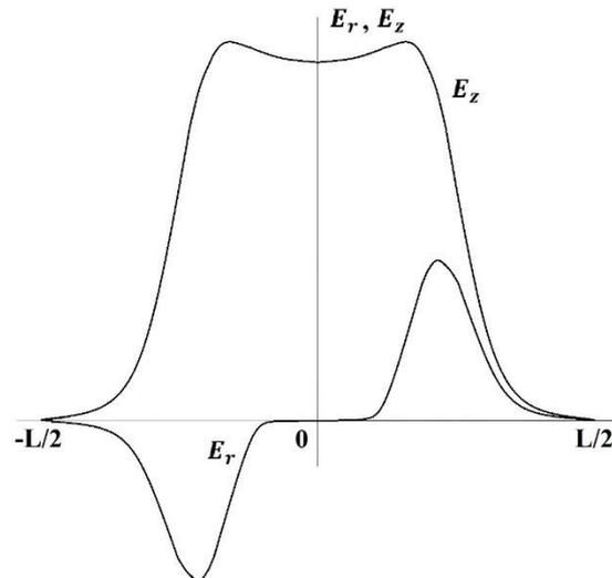
**Figure 3** Relative distribution of the longitudinal and radial components of the electric field in the aperture of the passage channel at a distance  $r \neq 0$  from the axis.
