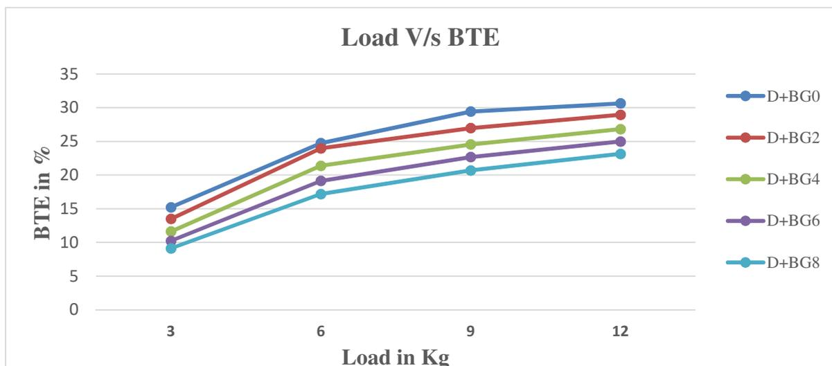
Graph 3 Variation in BTE with the Engine Load
