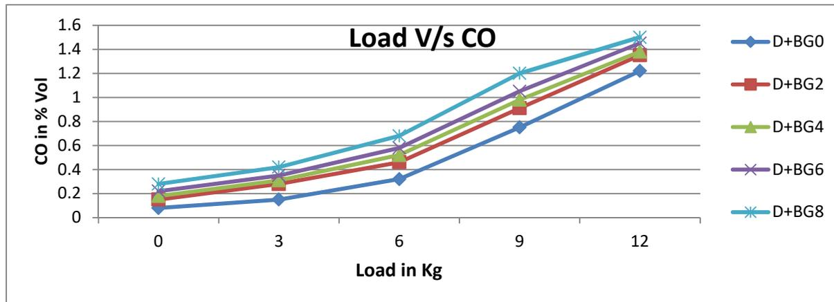
Graph 6.4 Variation in CO emission with the Engine Load
