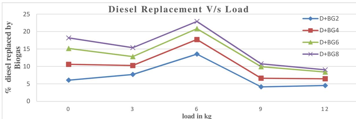
Graph 1 Variation in diesel replacement with the Engine Load
