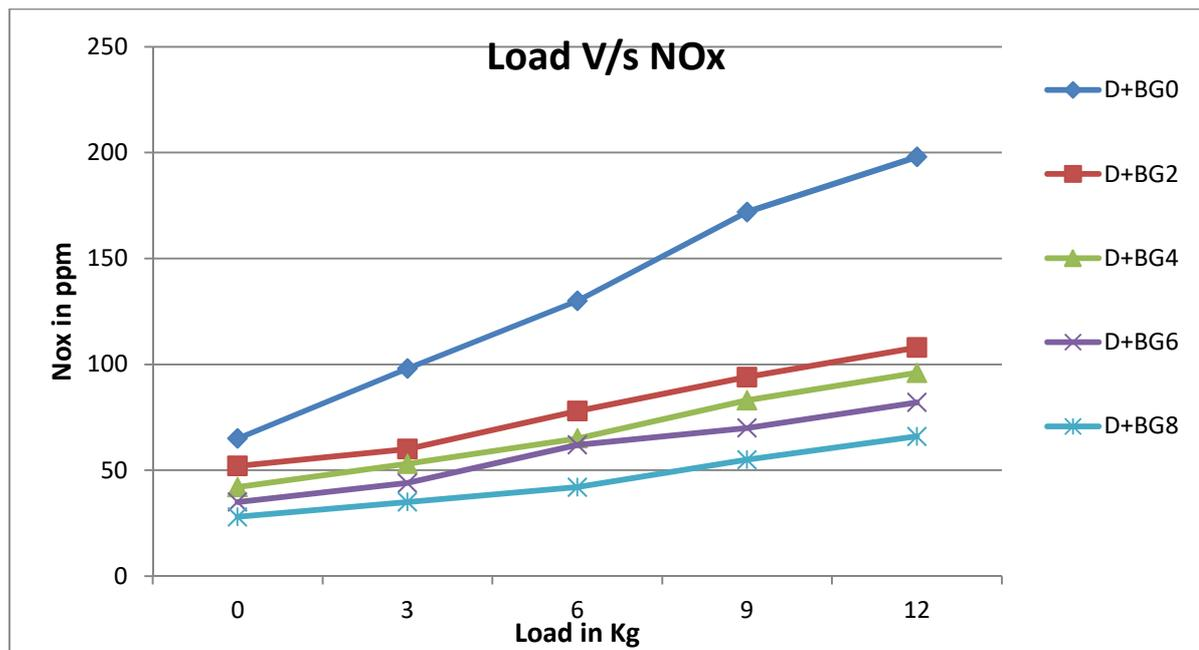
Graph 4.7 Variation in NO<sub>x</sub> emission with the Engine Load
