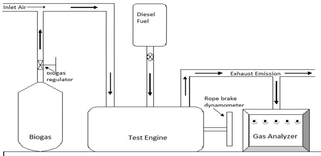
**Figure 3** Schematic diagram of experimental set-up
