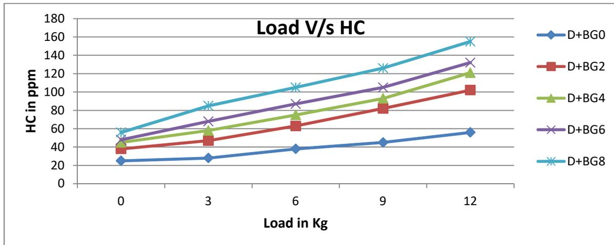
**Graph 4.6** Variation in HC emission with the Engine Load
