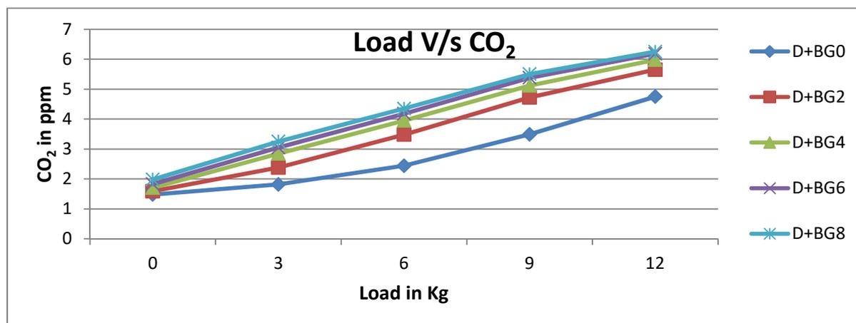
Graph 4.5 Variation in CO<sub>2</sub> emission with the Engine Load
