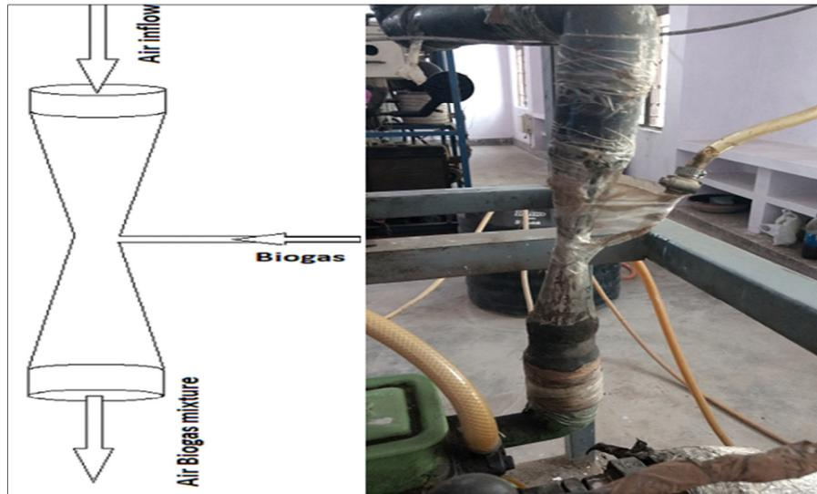
**Figure 2** Schematic and Actual Photograph of Inspirator System
