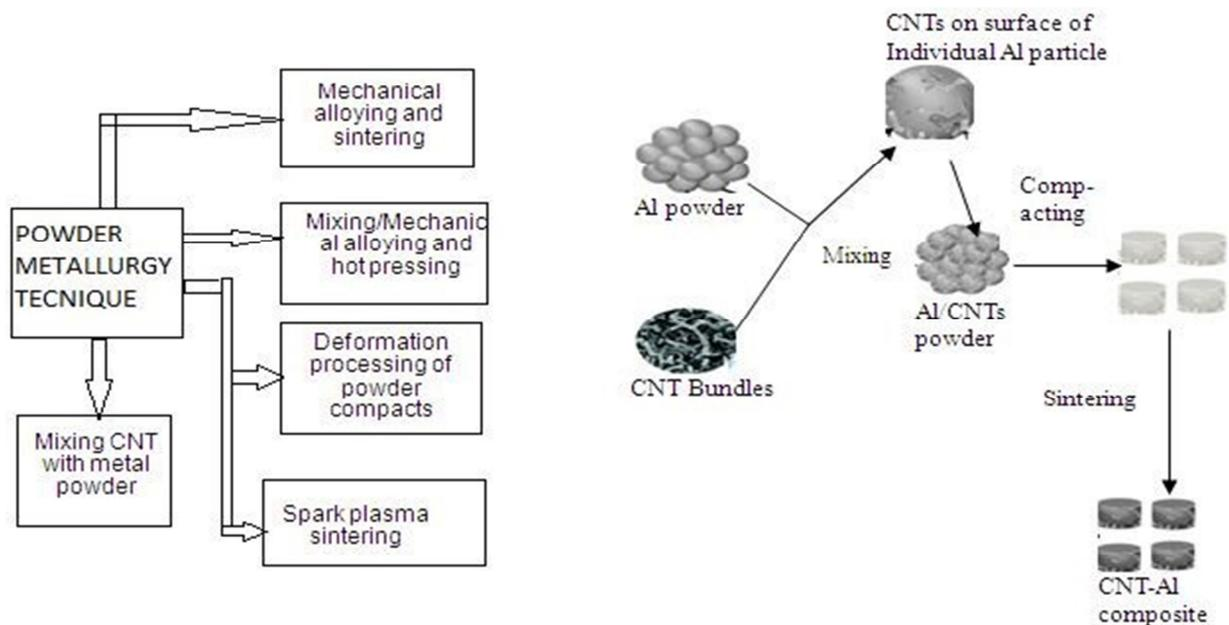
**Figure 1** Fabrication of carbon reinforced aluminium nano composite.
