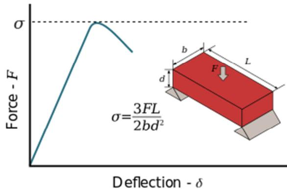
**Figure 2** Plot of Flexural strength to be measured.
