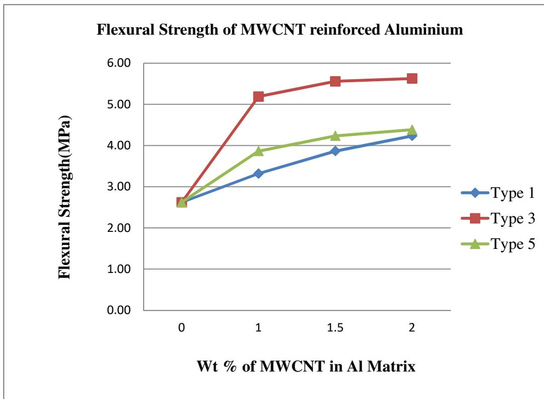
**Graph 1** Relation between weight percentage and flexural strength for types of aluminium composites used.
