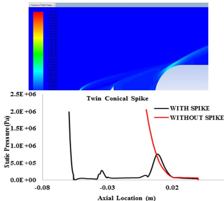
Figure 6 Pressure Distribution of Twin -Spike
