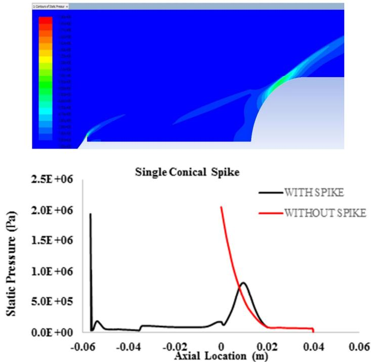
**Figure 2** Pressure Distribution over a Single Conical Spike
