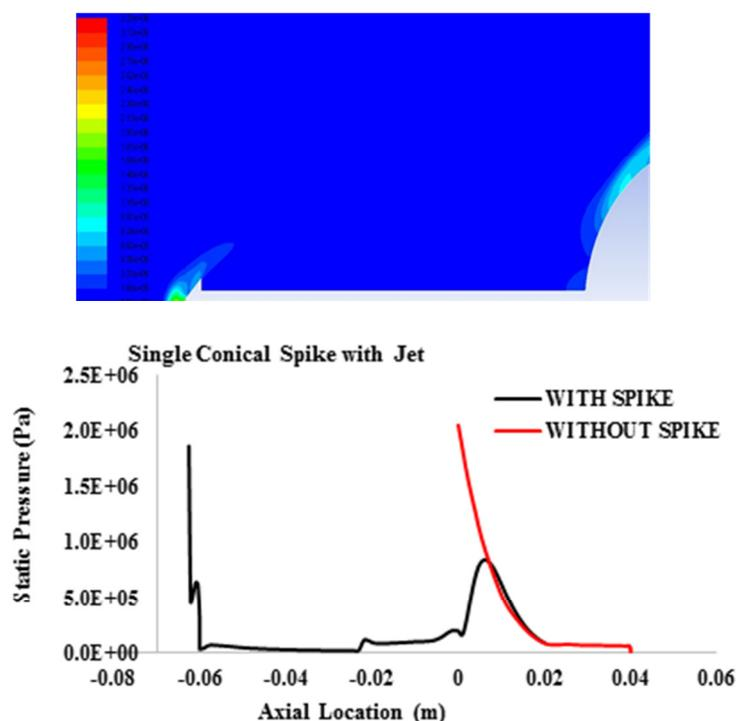
Figure 4 Pressure Distribution of Single Conical Spike with Jet
