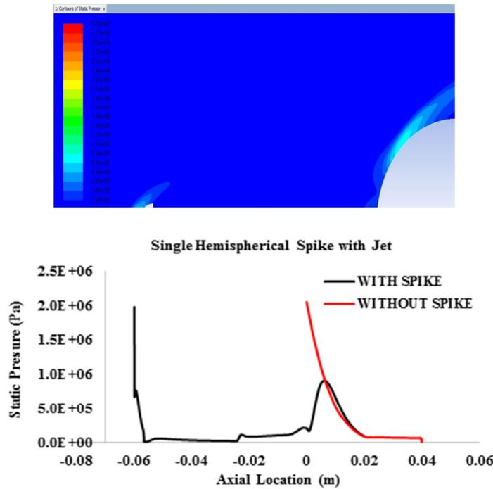
Figure 5 Pressure Distribution of Single Hemispherical Spike with Jet
