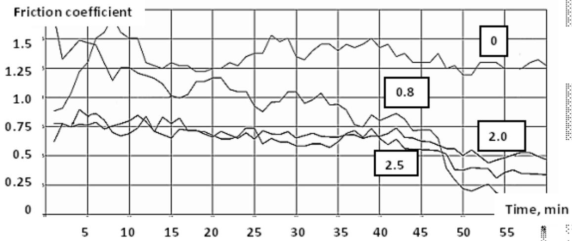
**Figure 2** Friction coefficients during wear testing of steel, grade 45 after nitriding in ammonia at 585°C in 3 h: curve 1 – conventional nitriding, curves 2-4 – nitriding with application of CuO film (numbers near curves – film thickness).
