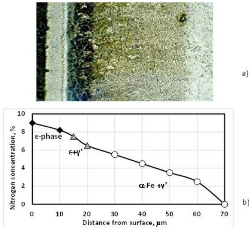
**Figure 1** Microstructure of steel, grade 40Kh after nitriding at 585°C in 3 h with preliminary applied copper oxide film (a) and nitrogen concentration profile over the thickness of nitrided layer (b).
