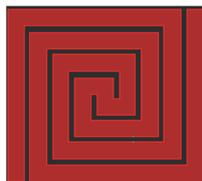
**Fan shape (figure 4):** A modified double spiral shape results in a fan shape geometry. The structure is later proved to be one of the best to obtain uniform temperature profile and less power consumption. Figure 4
