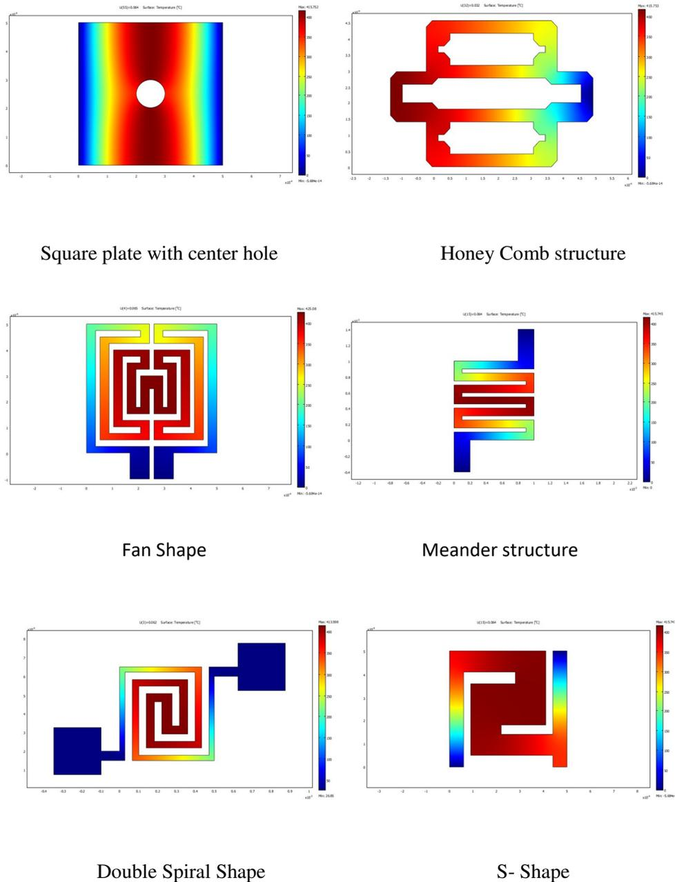
**Figure 8** Temperature profile of the microheater patterns
