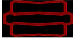
**S-Shape (figure.6):** One of the suitable structures for uniform temperature profile and lower power. But will be best for sensing film of small dimensions. Figure 6
