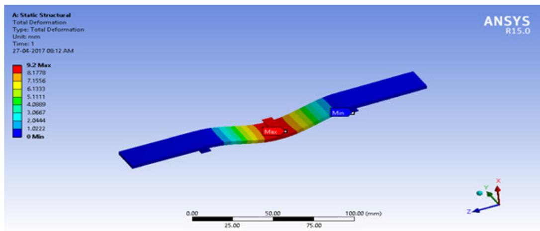
Figure 12 shows Total Deformation
