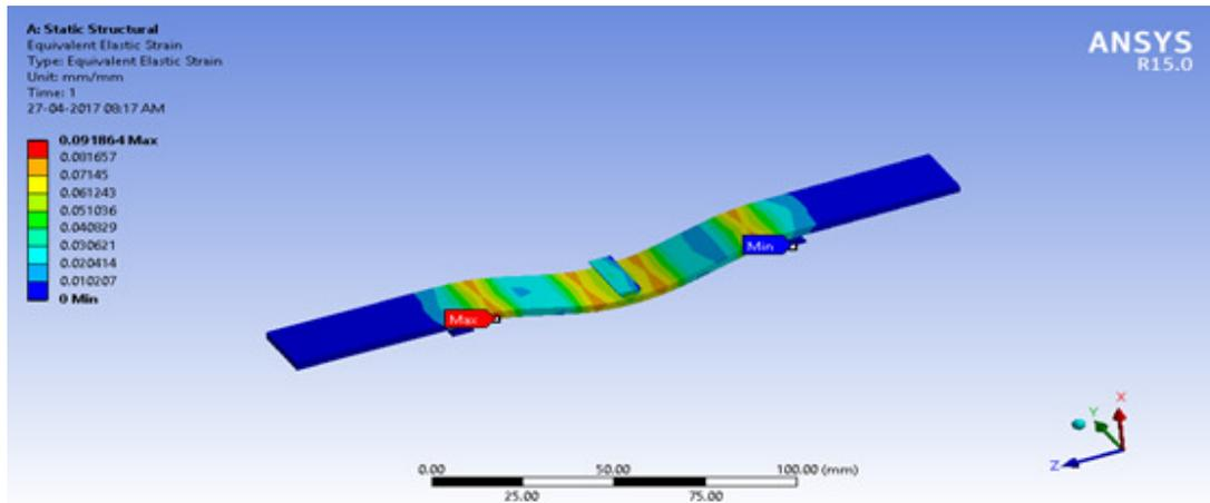
Figure 10 shows Equivalent Strain
