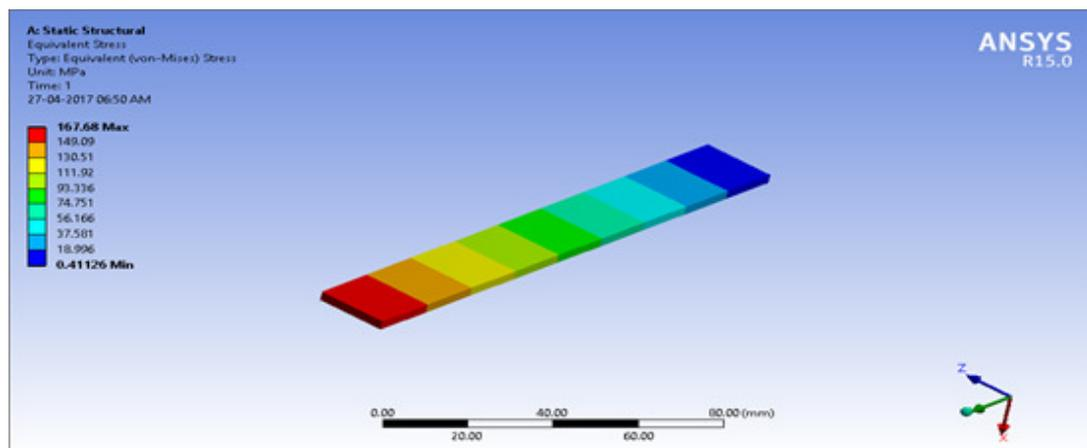
Figure 2 shows Von-Mises Stress
