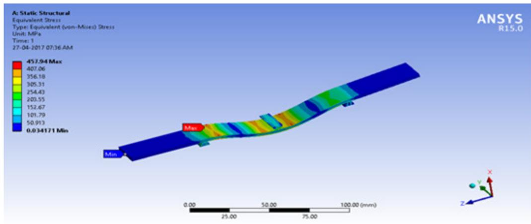
Figure 8 shows Von-Mises Stress
