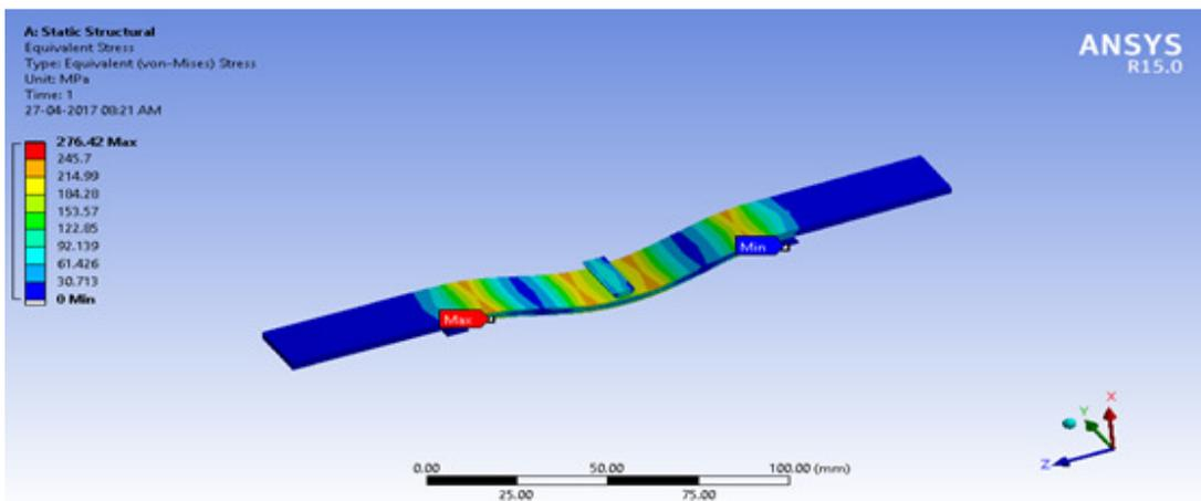
Figure 11 shows Von-Mises Stress
