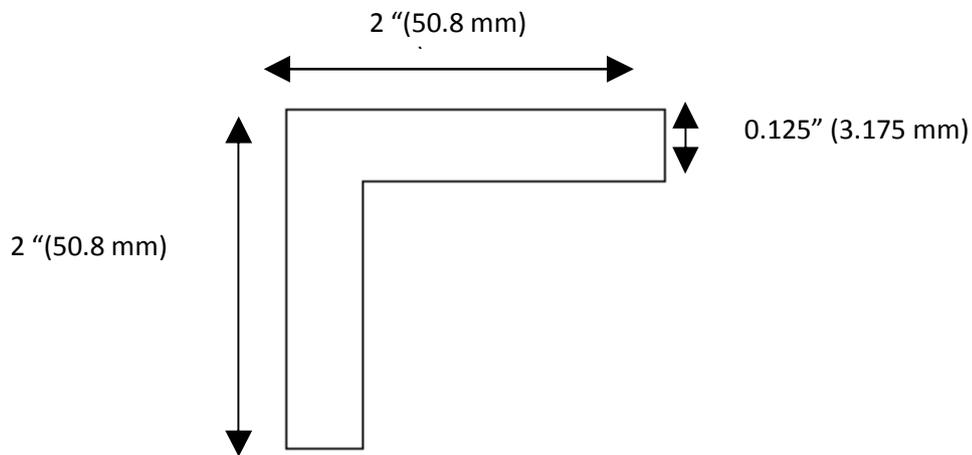
**Figure 2** L cross section
