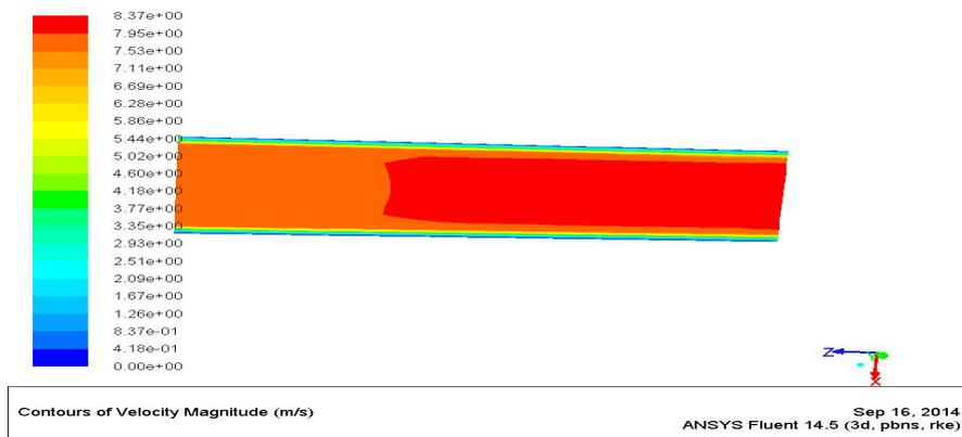
**Figure 7** shows Velocity contours smooth tube velocity  $Re=2300$
