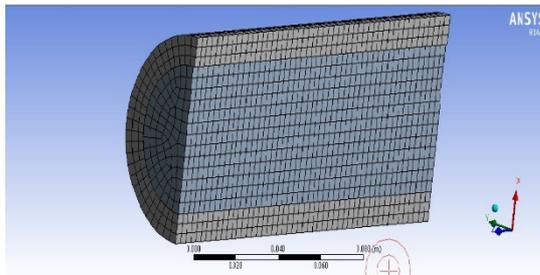
Fig 3 Shows CFD Meshing of Plain tube
