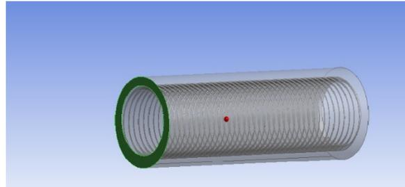
Fig 2 shows CFD Model of Internally Threaded tube
