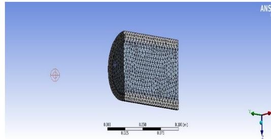
Figure 4 shows CFD Meshing of Internally threaded tube
