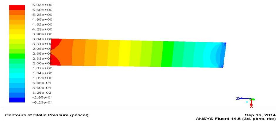
Figure 5 shows Pressure contours smooth tube velocity Re=2300
