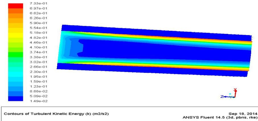
**Figure 6** shows Turbulence contours smooth tube velocity  $Re=2300$
