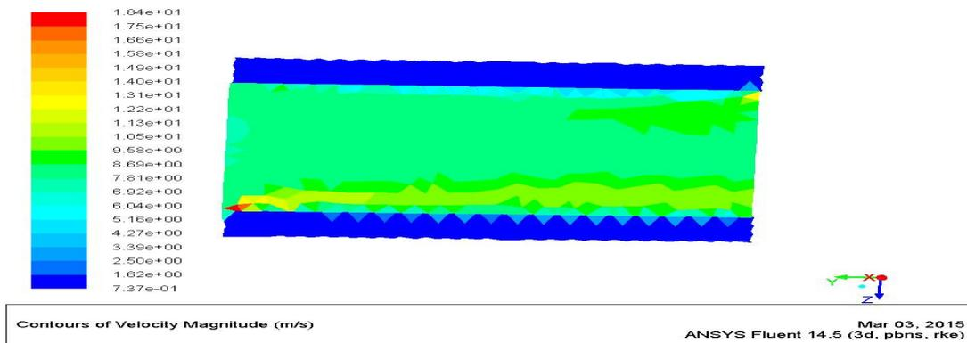
**Figure 3** shows Velocity contours internally threaded tube velocity  $Re=2300$
