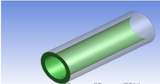
Fig 1 shows CFD Model of Plain tube
