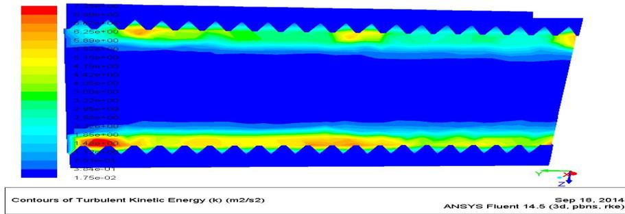
**Figure 9** shows Turbulence contours internally threaded tube velocity  $Re=2300$
