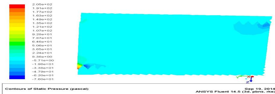
**Figure 8** shows Pressure contours internally threaded tube velocity  $Re=2300$
