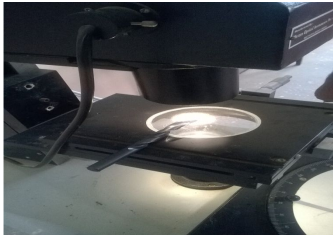
Figure 2 Carbide coated drill bit on profile projector
