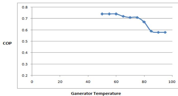
Above graph showing the variation of COP value with different temperatures at the heat generating unit of Ammonia water as a refrigerant.
