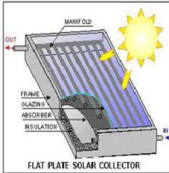
Figure 2 Flat plate collector parts
