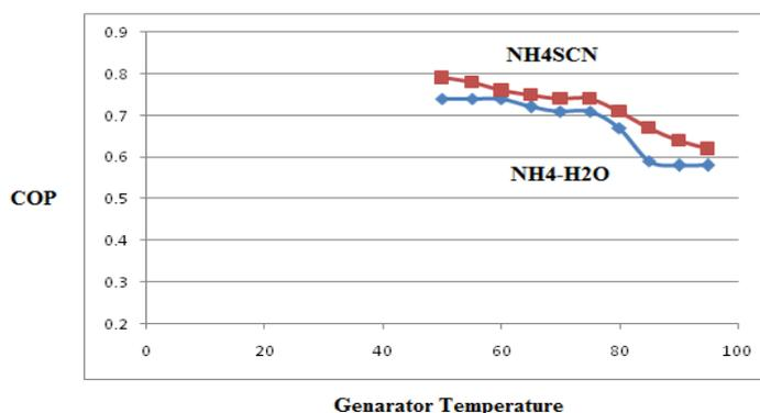
This is the graph showing you the comparison between Ammonia water and ammonium thiocyanate as a working pair and Conclude that improvement in the COP value is obtained ammonium thiocyanate as a working fluid.
