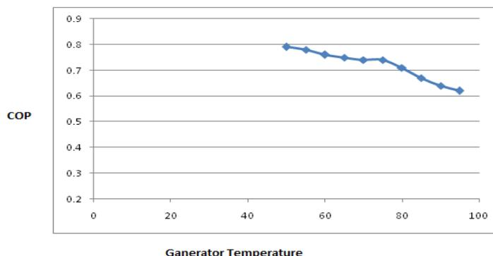
Above graph showing the variation of COP value with different temperatures at the heat generating unit of Ammonium thiocyanate as a refrigerant and this will give you the best COP value compared to the aqua ammonia solution.
