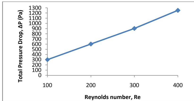
**Figure 5** Variations in total pressure drop with different values of Reynolds number
