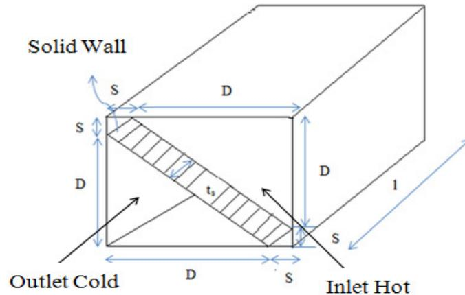
**Figure 1** Schematic of isosceles right triangular microchannel heat exchanger
