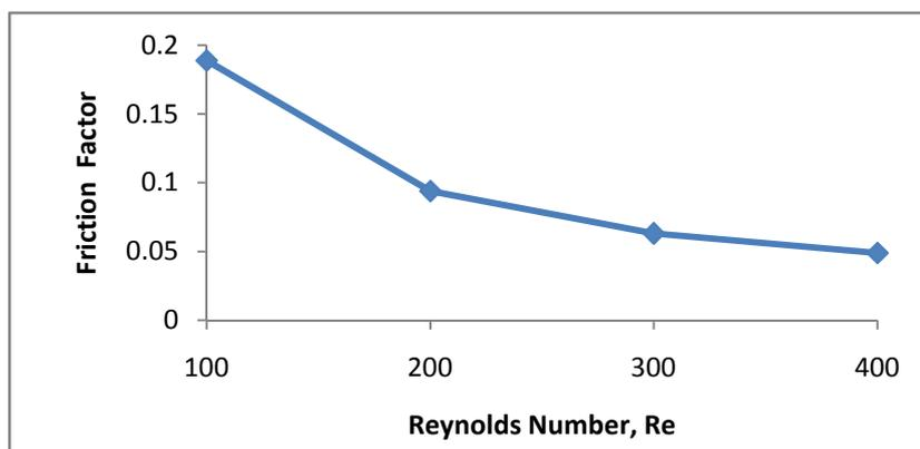
**Figure 6** Variation in friction factor with different Reynolds number
