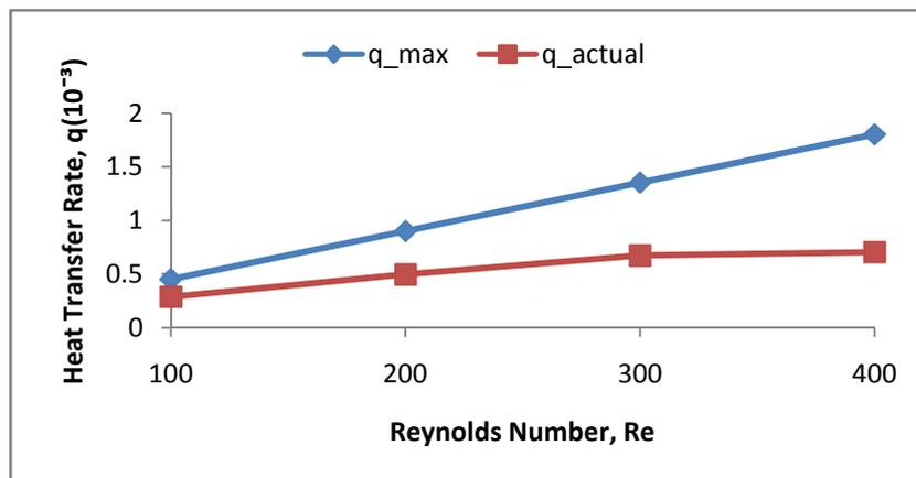
**Figure 4** Variation in heat transfer rate with different values of Reynolds number
