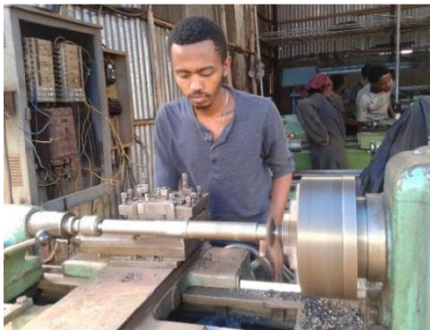
Figure 4 Shaft during manufacturing
