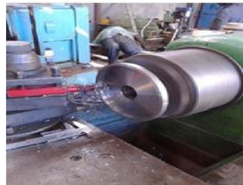
Figure 5 casing disk during manufacturing
