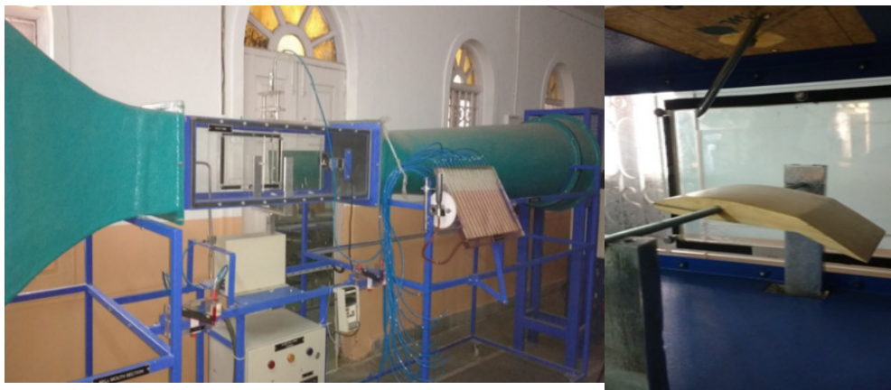
Figure 16 Wind tunnel testing setup
