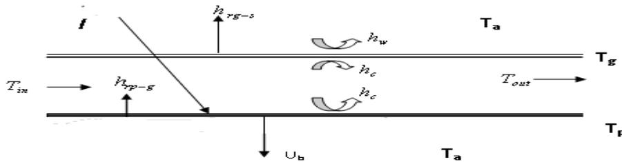
Figure 2 Energy balance on an absorber plate
