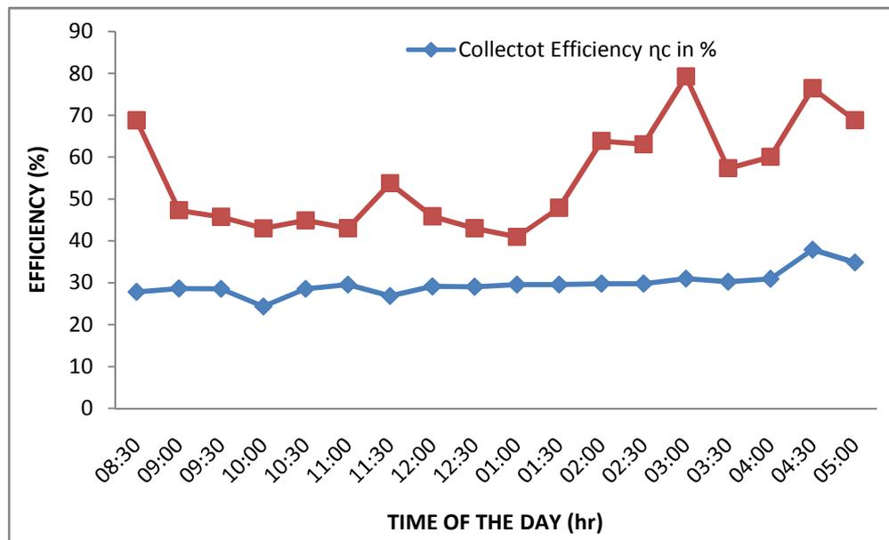
**Figure 5** Variation of efficiencies (Collector and Thermal) of the system w.r.t. time of the day
