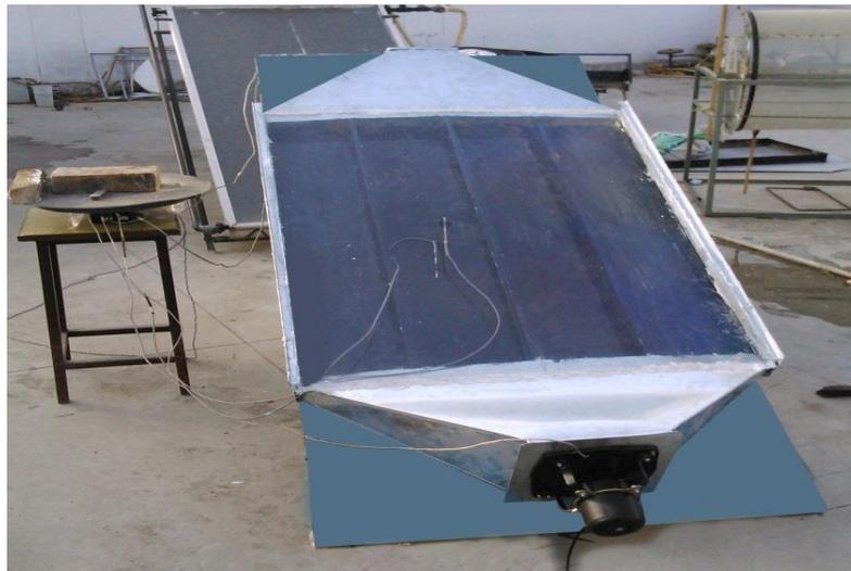
**Figure 1** Photograph of the experimental set up of the solar air heater.
