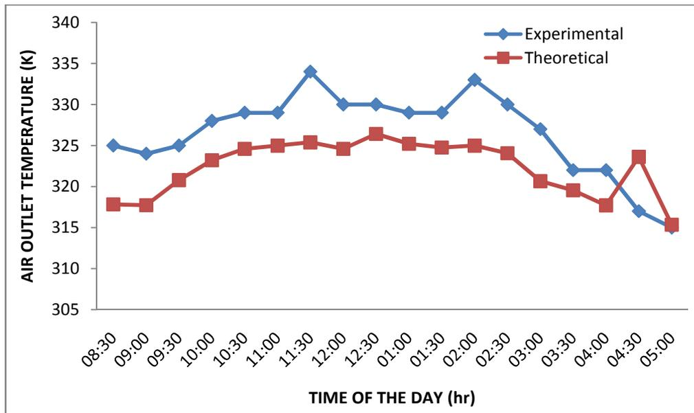
**Figure 4** Variation of air outlet temperature of the system w.r.t. time of the day
