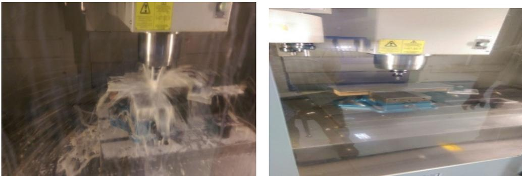
**Figure 11** Fabrication of Aluminium Chassis in CNC Machine
