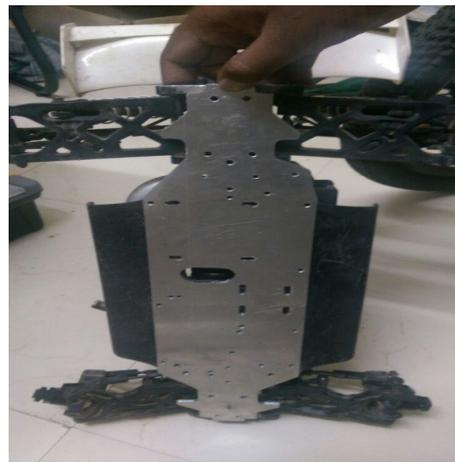
**Figure 12& 13** Fabricated Aluminum Chassis
