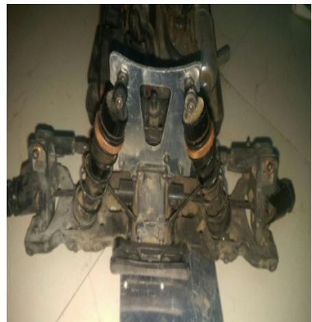
**Figure 15** Aluminum Shock Tower
