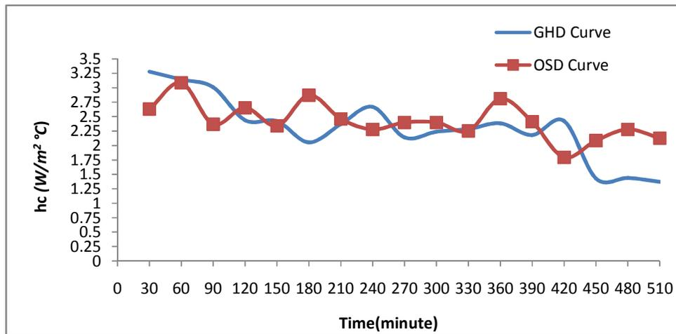
Fig. 8 Variation of Convective heat transfer coefficient ( $W/m^2 \text{ } ^\circ C$ ) Vs time
