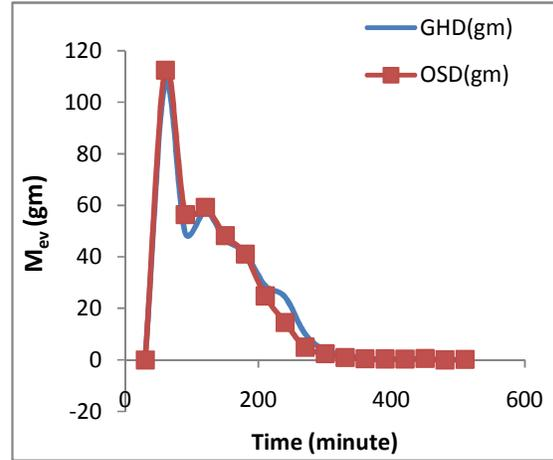
Fig. 7-variation of Moisture removal rate Vs time
