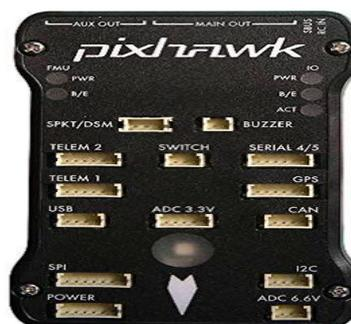
Figure 2 Pixhawk flight controller
