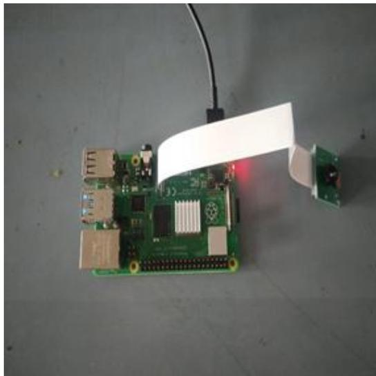
**Figure 8** Integration of raspberry pi and camera
