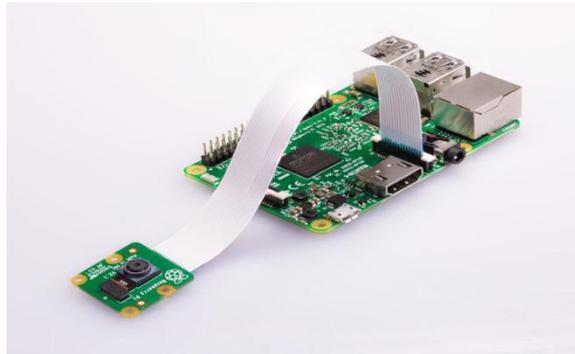
**Figure 3** Raspberry Pi and camera module
