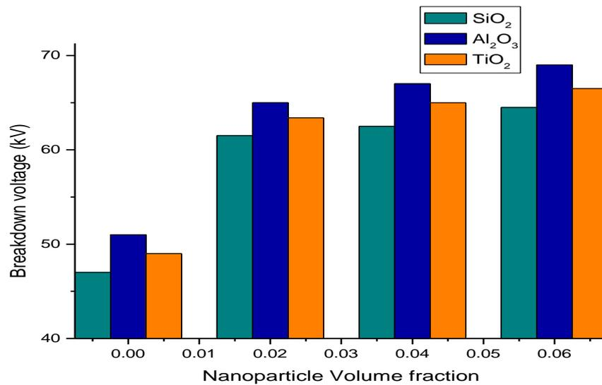
**Figure 5** breakdown strength of various nanofluids at different volume fractions
