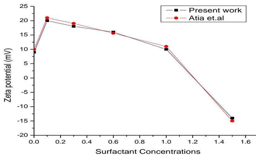
**Figure 6** Validation of zeta potential for  $\text{TiO}_2$  nanofluids [2].
