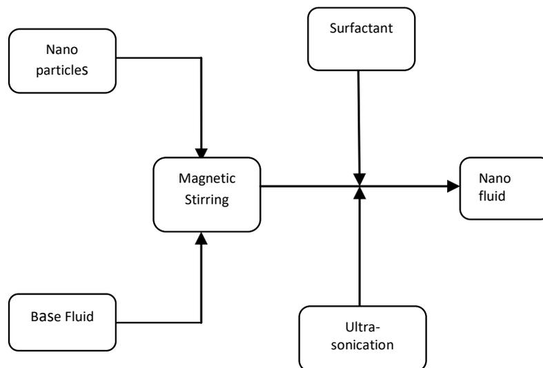
**Figure 1** Sequence of operations in preparation of nanofluids.
