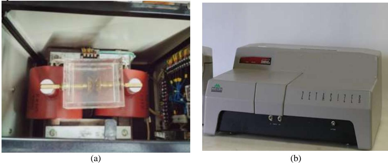
Figure 3 (a) Dielectric breakdown voltage measurement device (b) Zetasizer
