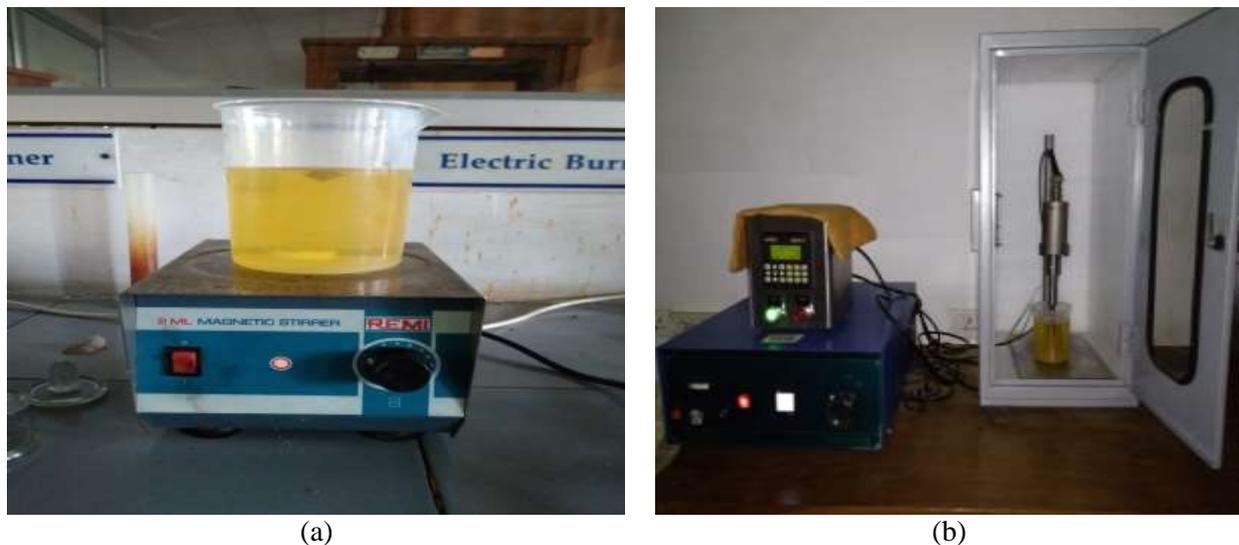
**Figure 2** Pictorial of (a) Magnetic stirrer (b) Ultrasonic Sonicator
