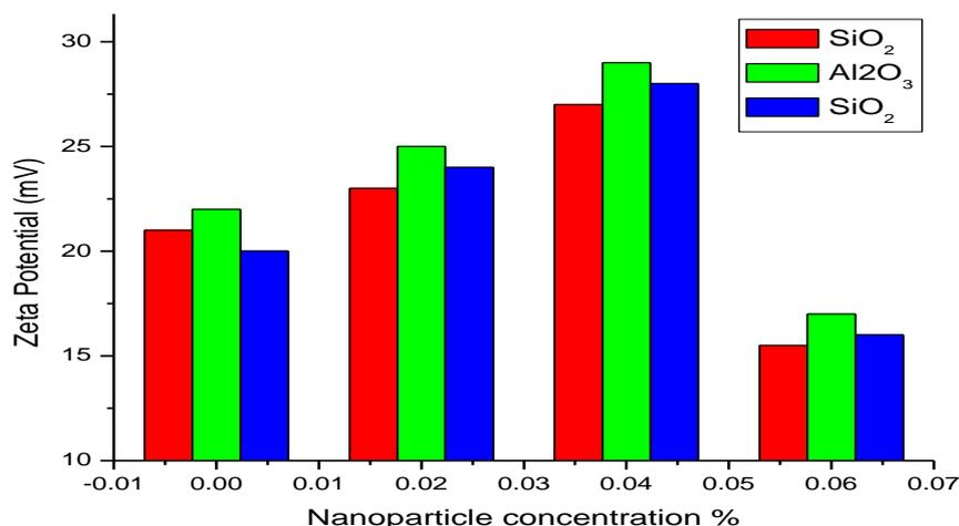
**Figure 7** Comparison of zeta potential values for various nanoparticle concentration.
