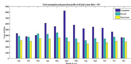
**Figure 3** Total consumption and generation profile(off-grid system)
