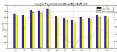
**Figure 4** Comparison of PV generation in mono-crystalline & multi-crystalline PV module
