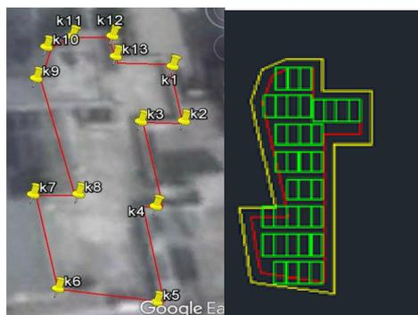
**Figure1** PV system design using 1(a) Google earth, and 1(b) AutoCAD software
