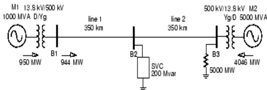
A 1000 MW hydraulic generation plant (M1) is connected to a load center through a long 500 kV, 700 km transmission line. The load center is modeled by a 5000 MW resistive load. The load is fed by the remote 1000 MVA plant and a local generation of 5000 MVA (plant M2).
