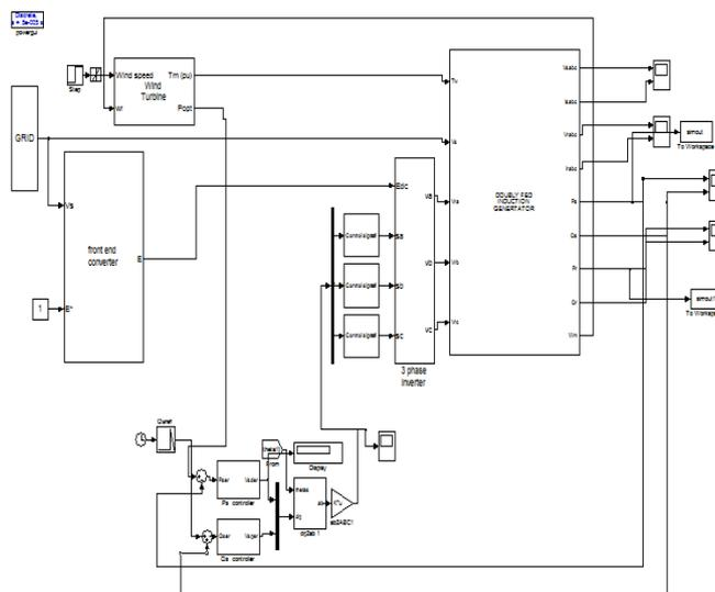
Figure 1 Simulation block diagram of DFIG
