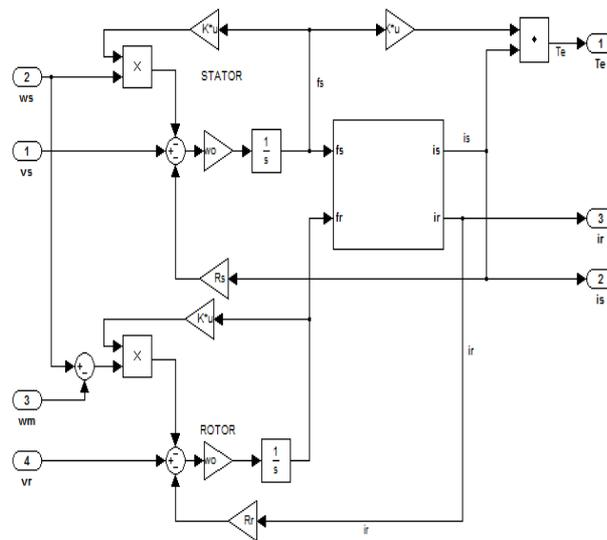
**Figure 2** Dynamic model of induction machine in arbitrary reference frame
