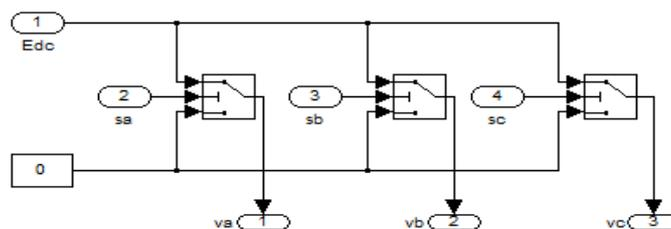
**Figure 4** Simulink diagram for rotor side converter
