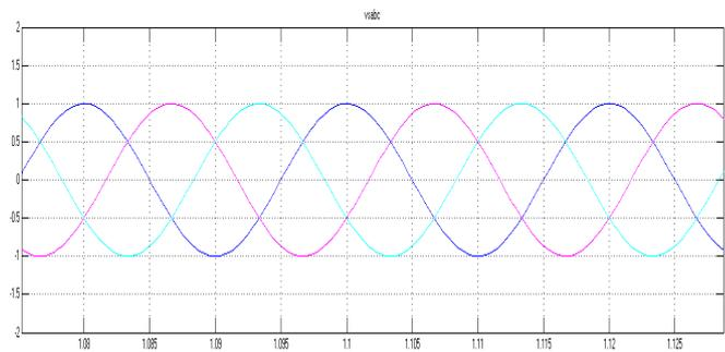
**Figure 6** Three phase rotor voltage.
