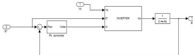
**Figure 3** Simulink diagram for Grid side converter
