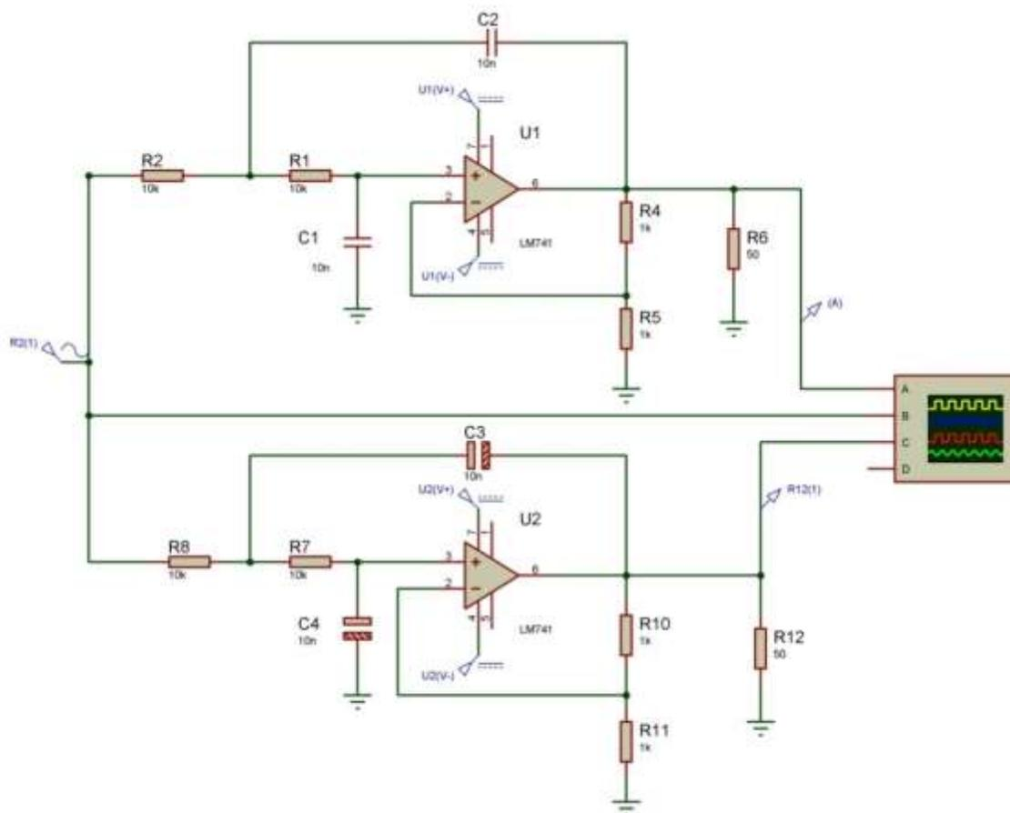
**Figure 1** Circuit design of the Butterworth low pass filter
