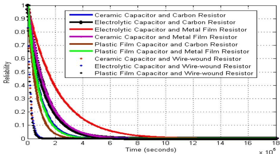
**Figure 5** Reliability plot for different combination of RC network for Active Filters
