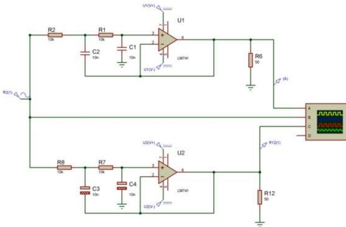
**Figure 2** Circuit design of the low pass Chebyshev filter
