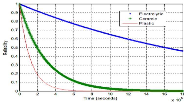
**Figure 3** Reliability plot for the various types of capacitors
