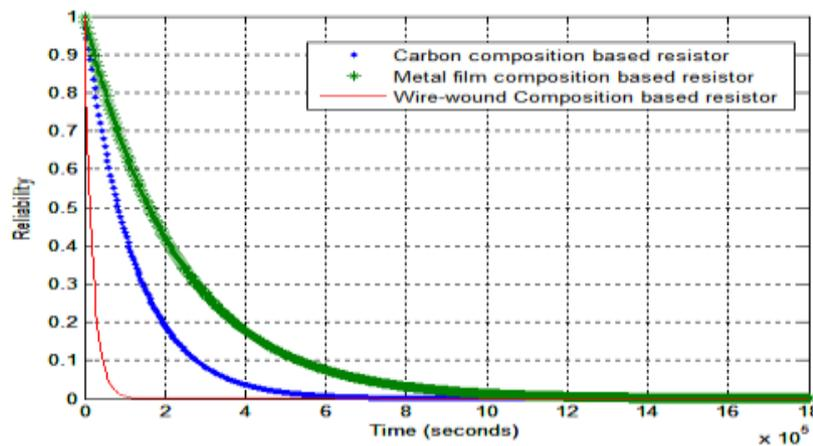
**Figure 4** Reliability plot for various composition based resistors
