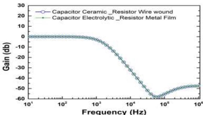
**Figure 7** The frequency response of the low pass Chebyshev filter for the two different combinations of the resistors and capacitors
