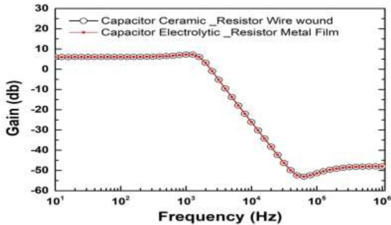
**Figure 6** The frequency response of the Butterworth low pass filter for the two different combinations of the resistors and capacitors
