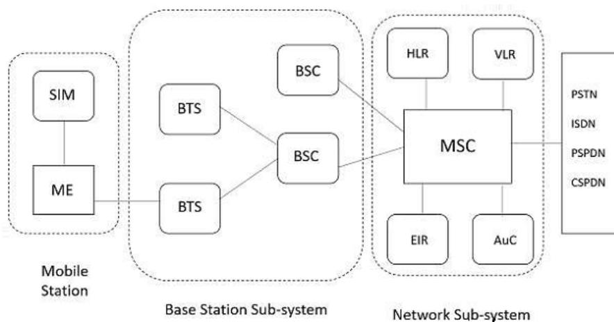
**Figure 1** Wireless infrastructure and components.
